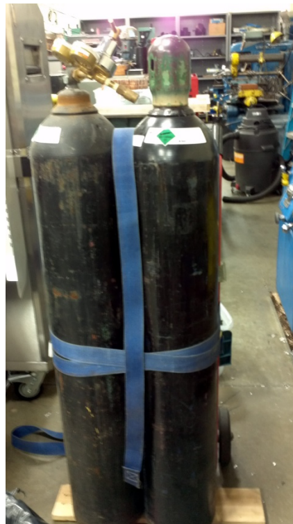
Figure 14: Nitrogen cylinder with regulator.
