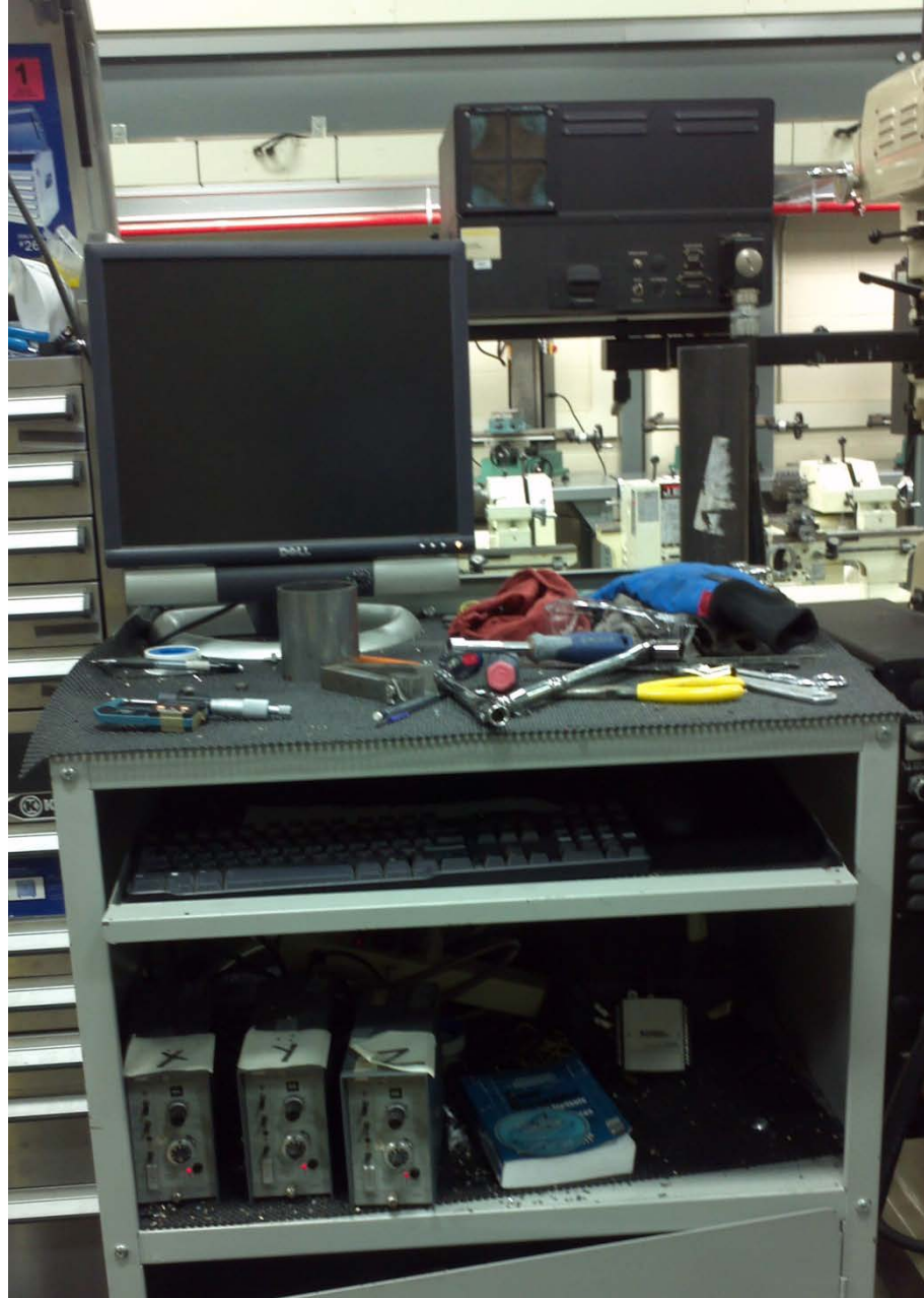
Figure 29: Data processing station containing charge amplifiers, DAQ, a PC with LabVIEW 8.2 software.
