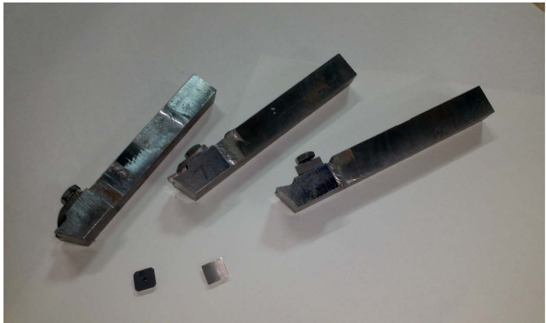
Figure 32: Three different tool holders with different rake angles machined in AISI 4140 Steel stock.
