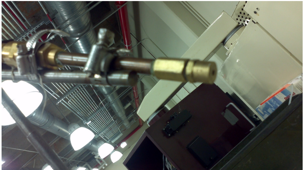
Figure 16: Nozzle supplying the coolants at the point of cutting.
