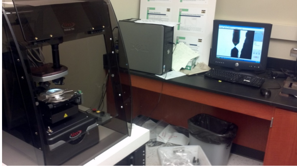
Figure 34: Surface profilometer with the computer screen in the background showing the scanning profile
