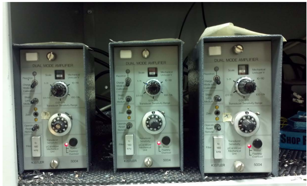
Figure 19: Kistler Model 5004 Charge Amplifiers
