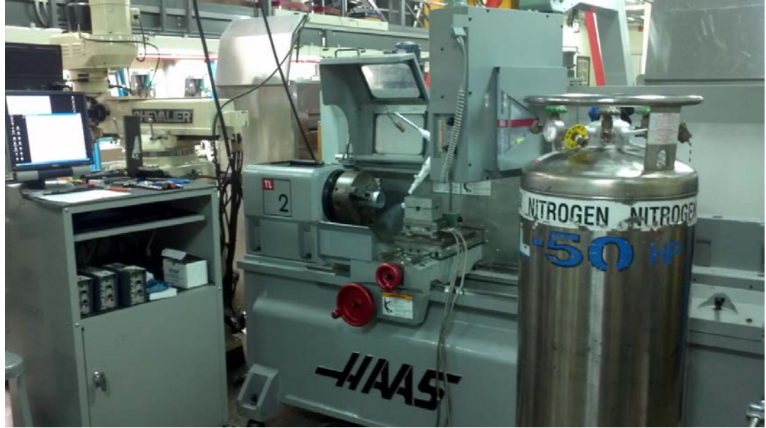
Figure 33: Example of a fully constructed orthogonal tube turning apparatus with liquid nitrogen cutting environment.
