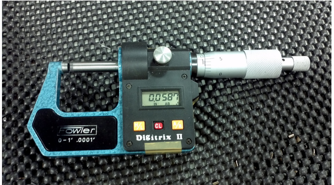
Figure 21: Fowler Digitrix II 0-1" Micrometer.
