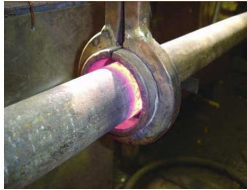
Figure 11 Induction welding operation
