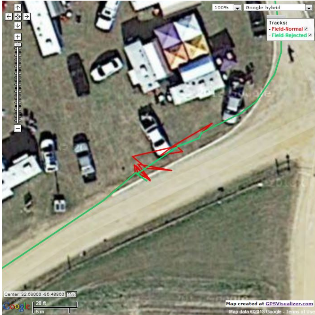
Figure 6.4: Comparison of position estimate with and without rejected signals.
