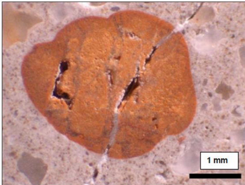
Figure 3.15. Cracks with alkali-silica gel in peripheral region of chert and cracked cement paste containing white ettringite deposits (WJE 2010)
