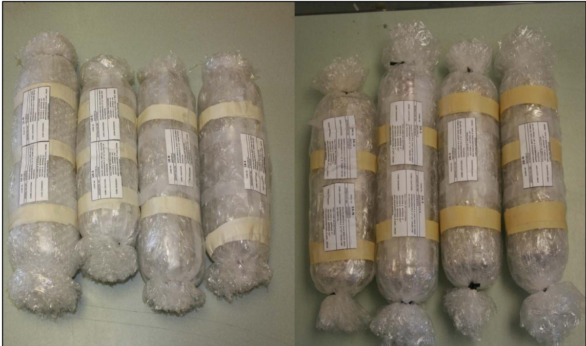
Figure A. 8. Wrapping of core samples
