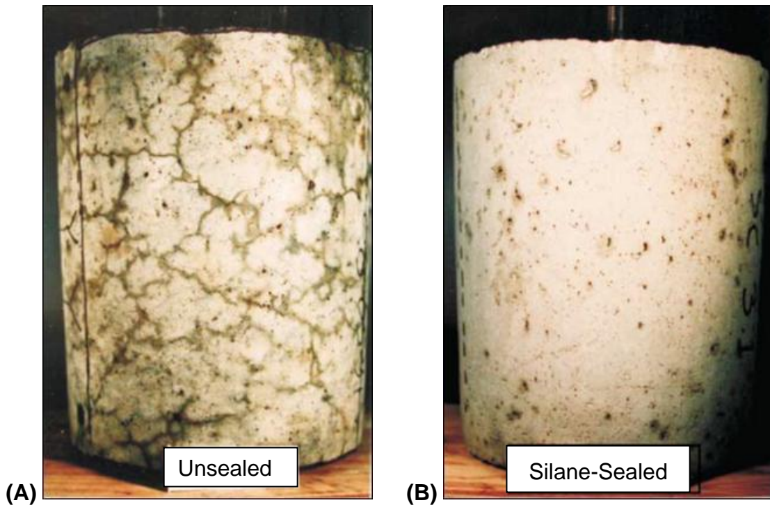
Figure 2.12. (A) Unsealed and (B) silane-sealed air-entrained concrete cylinders subjected to exposure cycle C4, after 1.5 years
