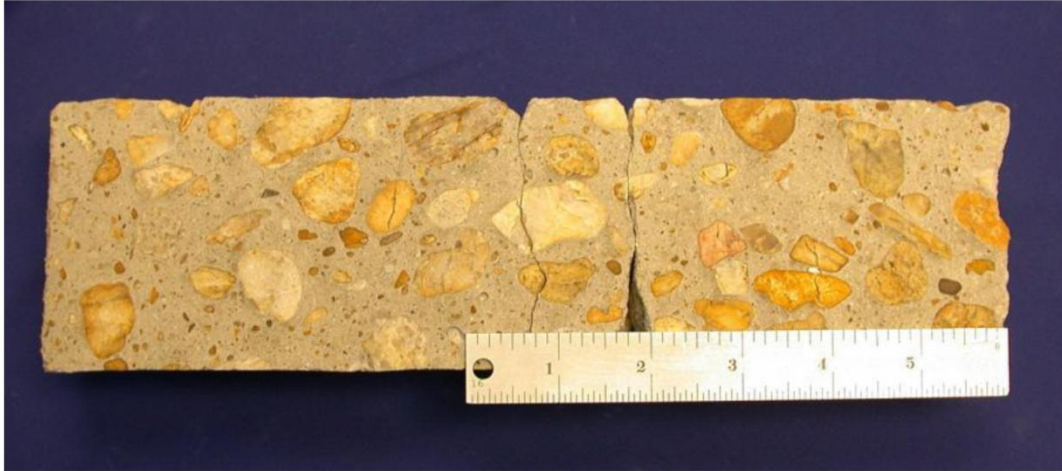
Figure 1. Lapped longitudinal cross section of Core 1A-N. Outside end of core is on left.
