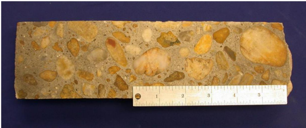
Figure 4. Lapped longitudinal cross section of Core 1B-S. Outside end of core is on left.
