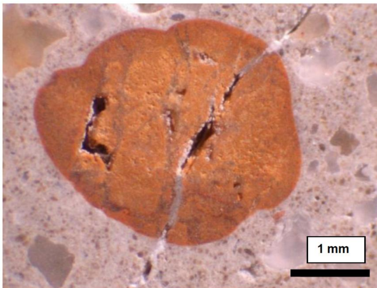
Figure 14. Wider cracks in chert particle are filled with ASR gel in peripheral region of particle. Cracks in paste contain white ettringite deposits.
