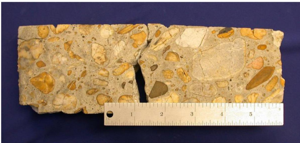
Figure 2. Lapped longitudinal cross section of Core 1A-S. Outside end of core is on left.
