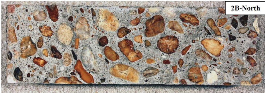
Figure 1. Polished concrete sections from the Gibb Graves Bridge, Wetumpka, Alabama.
