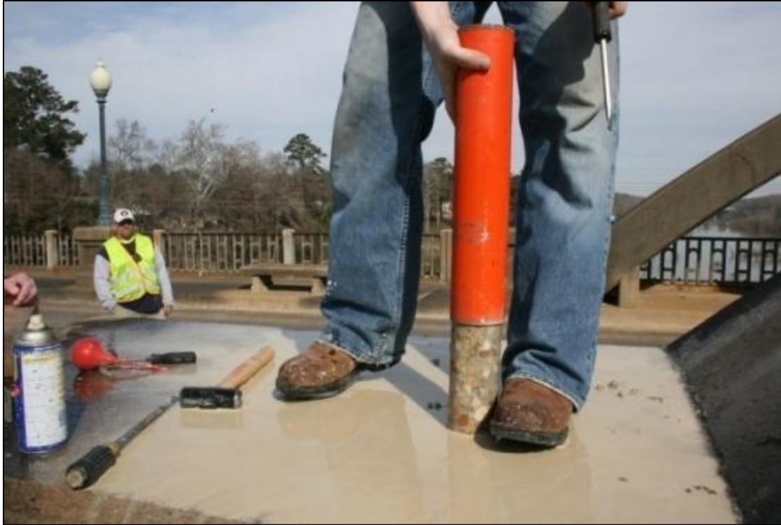
Figure A. 6. Extraction of core samples
