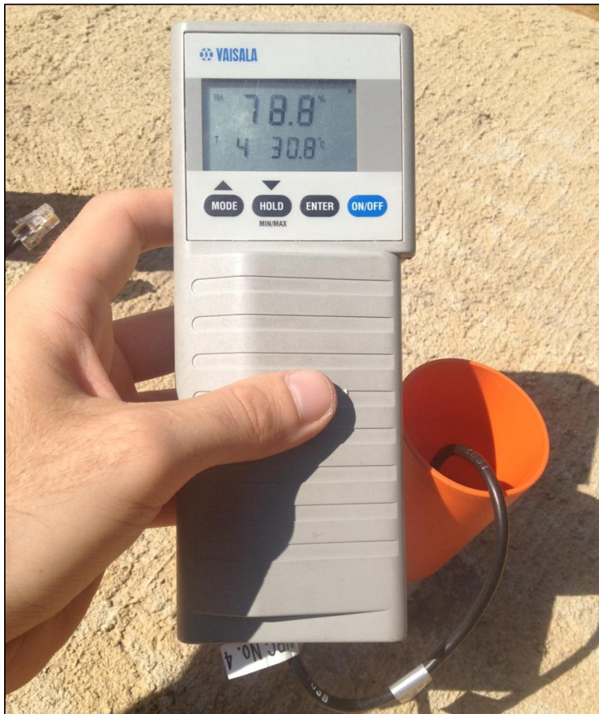
Figure 5.8. Measuring temperature and RH with indicator
