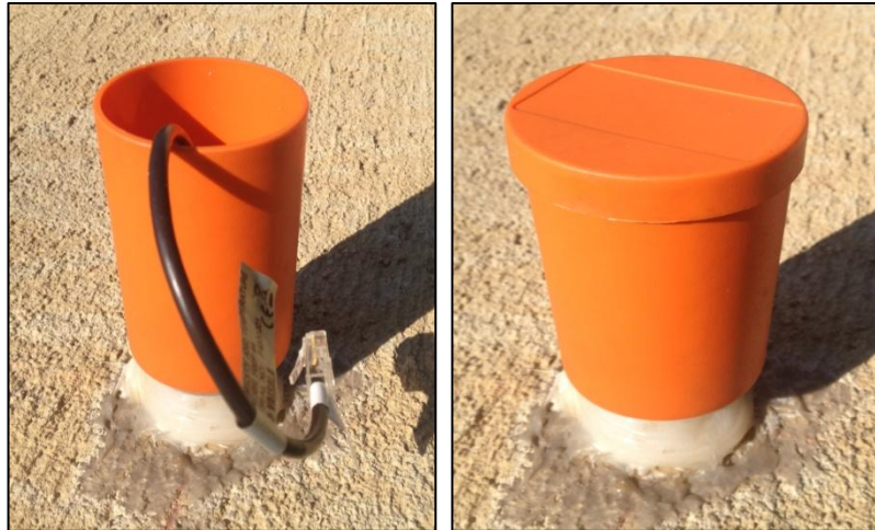
Figure 5.7. Placing protective cup and lid over tube
