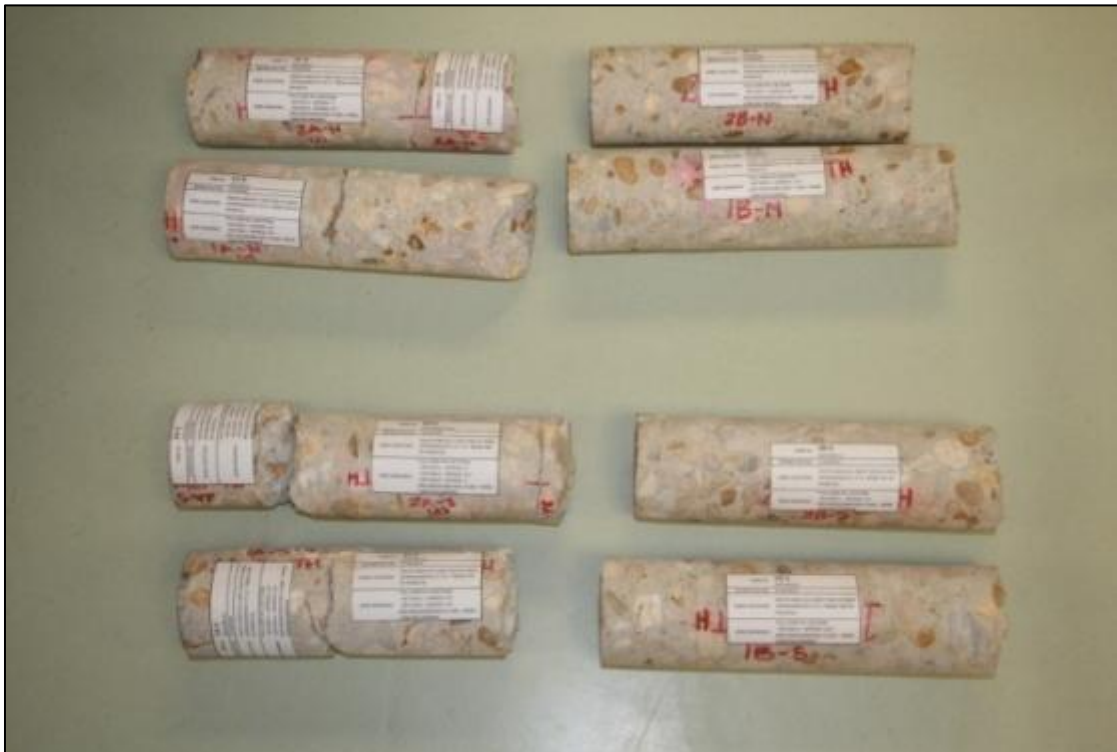
Figure A. 7. Labeling of core samples
