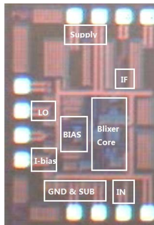
Figure 4.2. Die photo of the Blixer front end.
