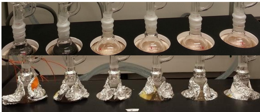
Figure 11. Efforts to avoid joint leakage showing aluminum foil tape (bottom) over traditional Parafilm (top).
