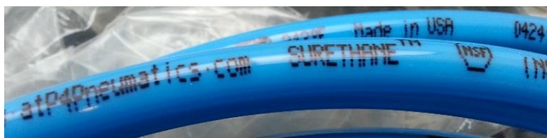
Figure 27. Originally acquired sample (29) polyurethane tubing (blue).
