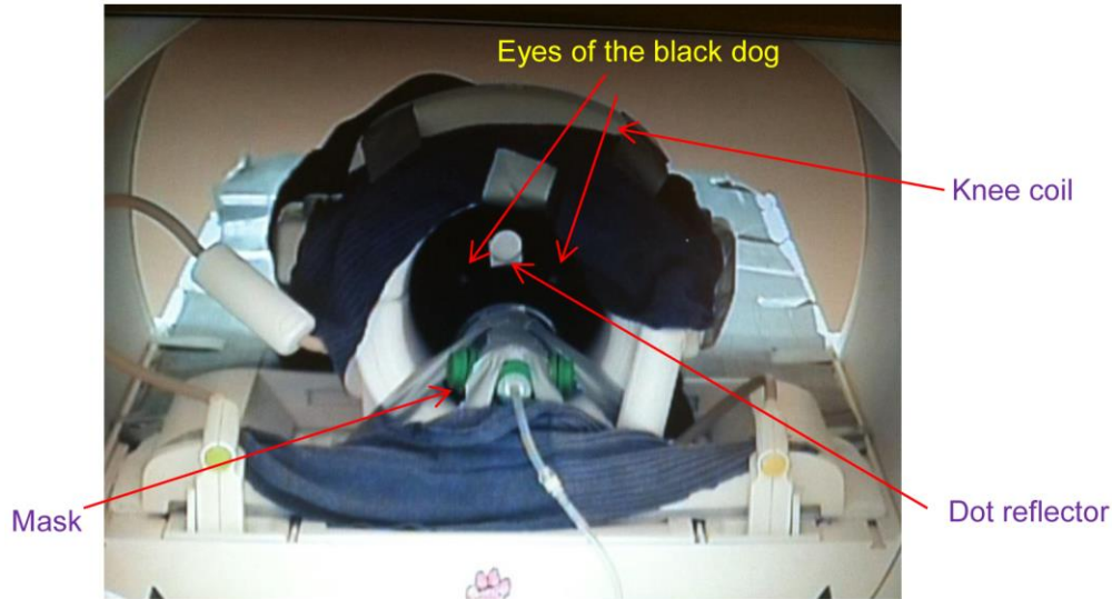
Figure 2.6 A black dog positioned with muzzle in mask for odorant delivery. The dot reflector is mounted to dog's head for motion tracking, the knee coil encompasses the dog's head and the mask is mounted on the front frame of the knee coil.
