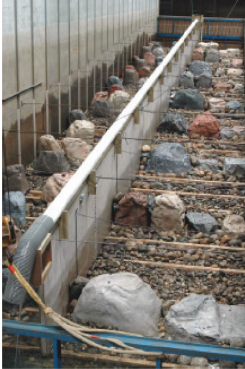
Test tracks with the perturbation boulders on the left and the rock weirs on the right.
