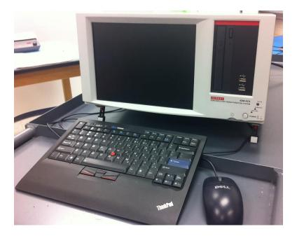
Figure A.7: Keithley 4200 (Semiconductor Characterization Systems) parameter analyzer.
