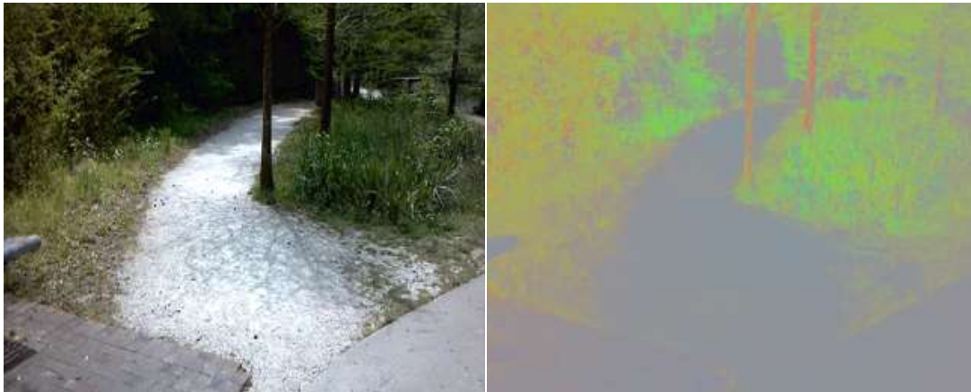
Figure 1, L-2 norm image comparison. Original image (left) compared to L-2 color normalized image (right).
