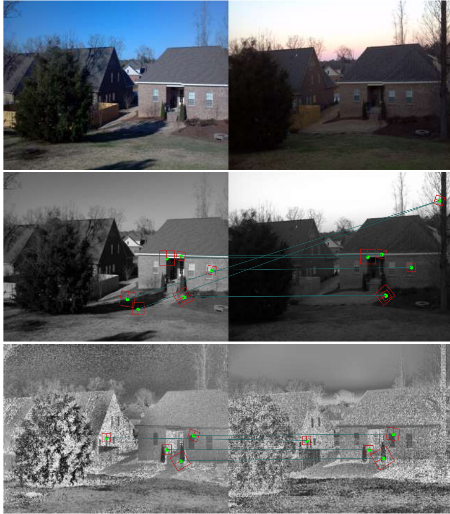
Figure 11, comparison of SIFT feature matching (2). Original image (top), grayscale image (middle), and log-chromaticity projected image (bottom). Note the incorrect matches from the grayscale images due to shadowing.
