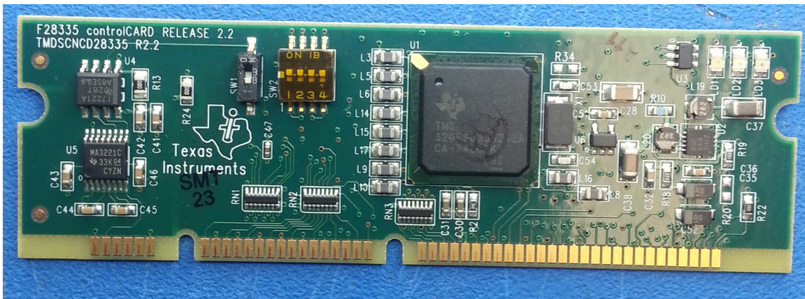
Figure 5.1: TI microcontroller used to control up to five buck phases
