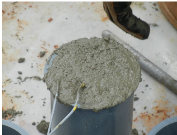
Figure 3-13: iButton Temperature Sensors in a 4x8 in. Cylinder
