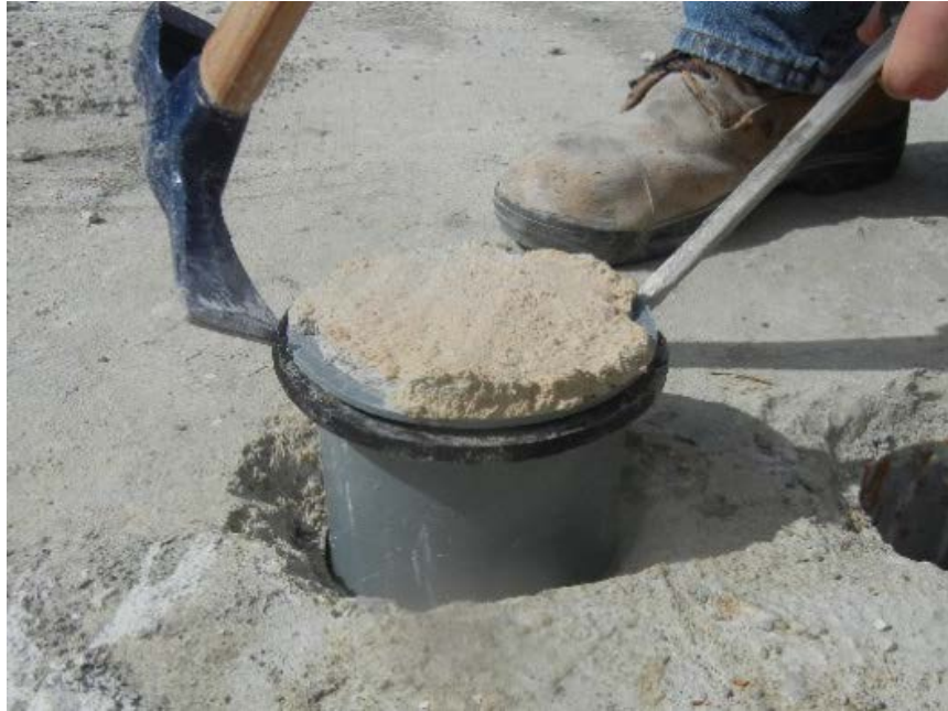
Figure 3-28: Removal of a Cast-In-Place Cylinder From a Slab
