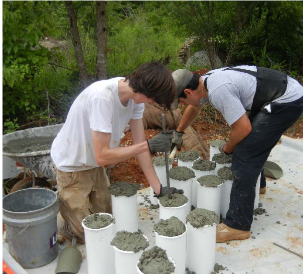
Figure 3-21: Making of 6×12 in. Molded Cylinders
