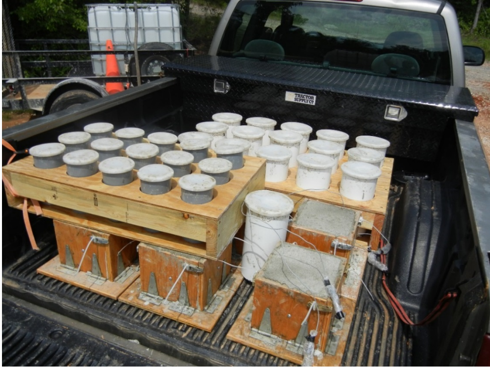
Figure 3-23: Molded Cylinders and Cubes Being Transported Back to AU Materials
