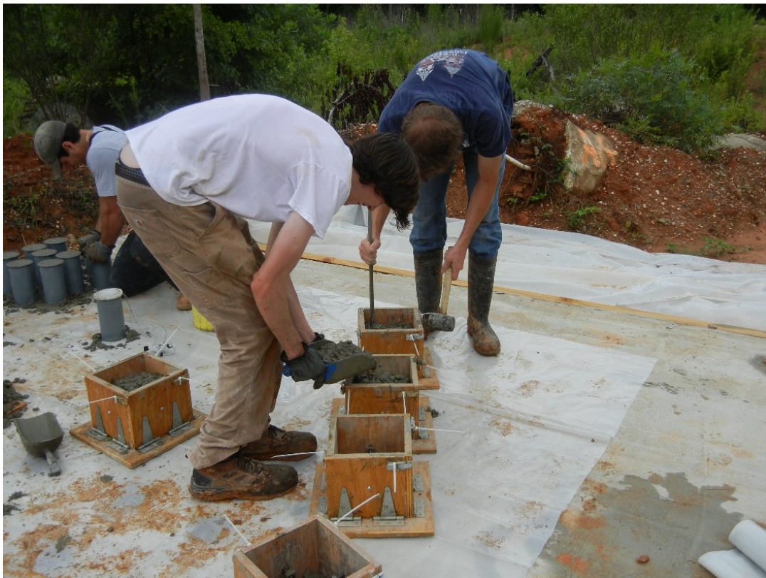
Figure 3-25: Making of the LOK-Test Pullout Calibration Cubes
