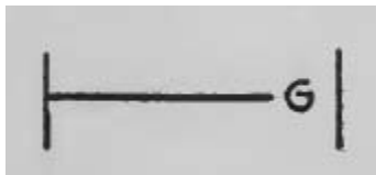
Figure 4.5 Chart Element Illustrating “Green Labor” cause of Idleness (Clark 1923)
