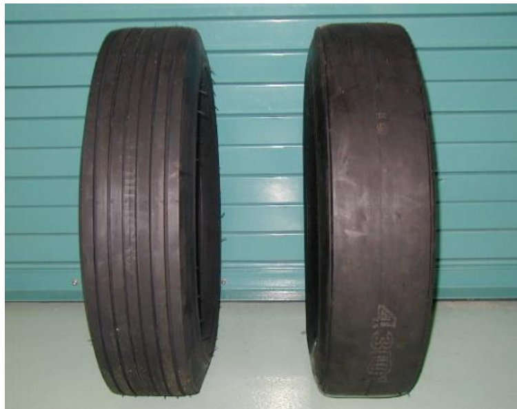
Figure 2.7: Photographic illustration of a ribbed (ASTM E501) versus smooth test tire (ASTM E524) (Choubane et al. 2006)
