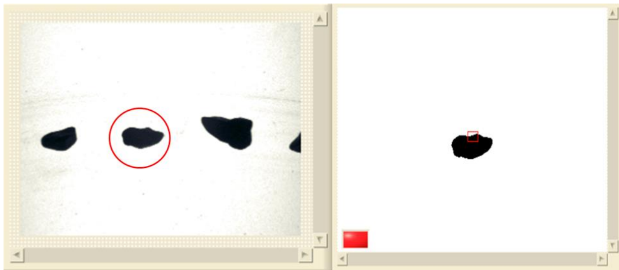
Figure 3.4: Example of rejected particle in the AIMS-II coarse aggregate analysis
