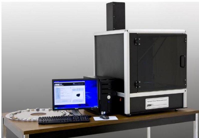
Figure 2.21: The second generation Aggregate Imaging Measurement System (Pine Instrument Company 2011)
