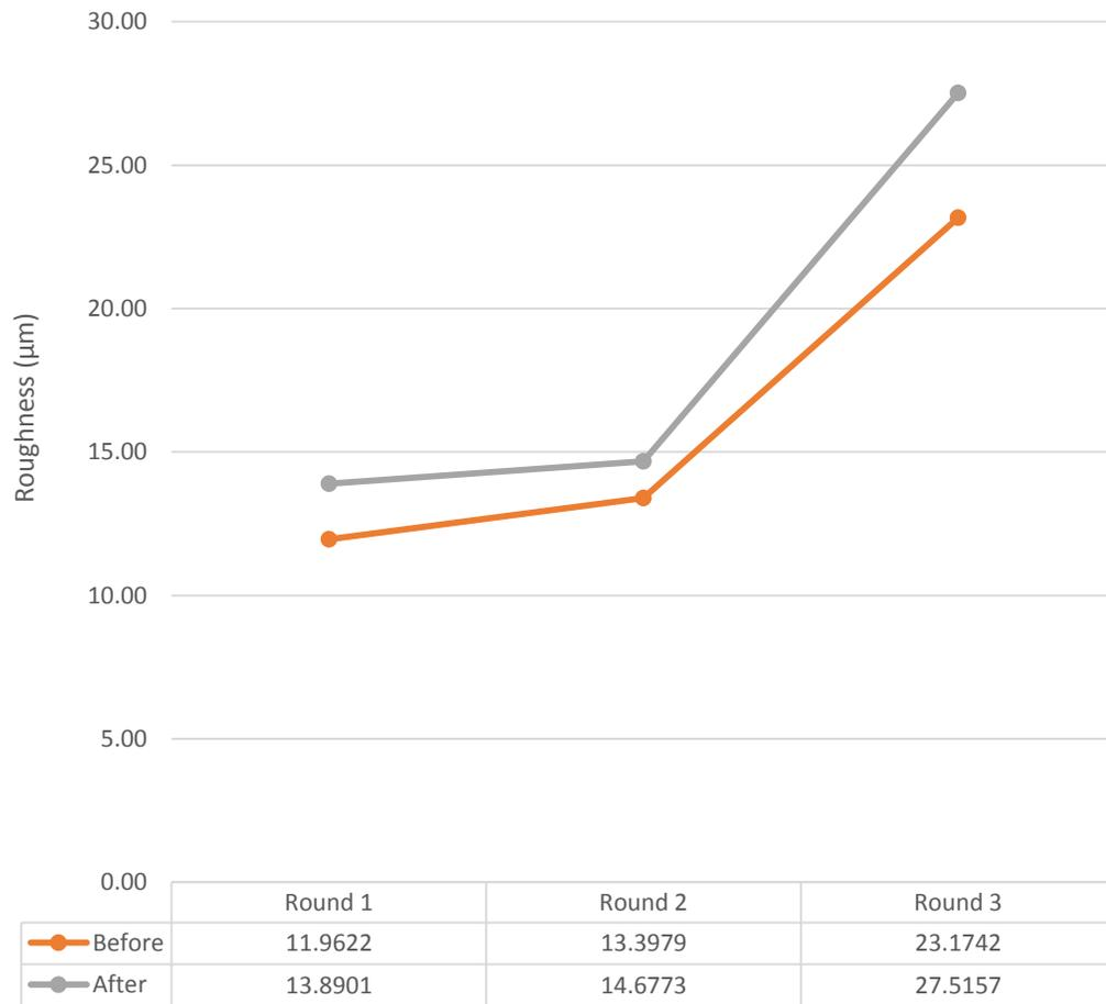
Figure 34. Surface roughness of FRP before and after the tests
