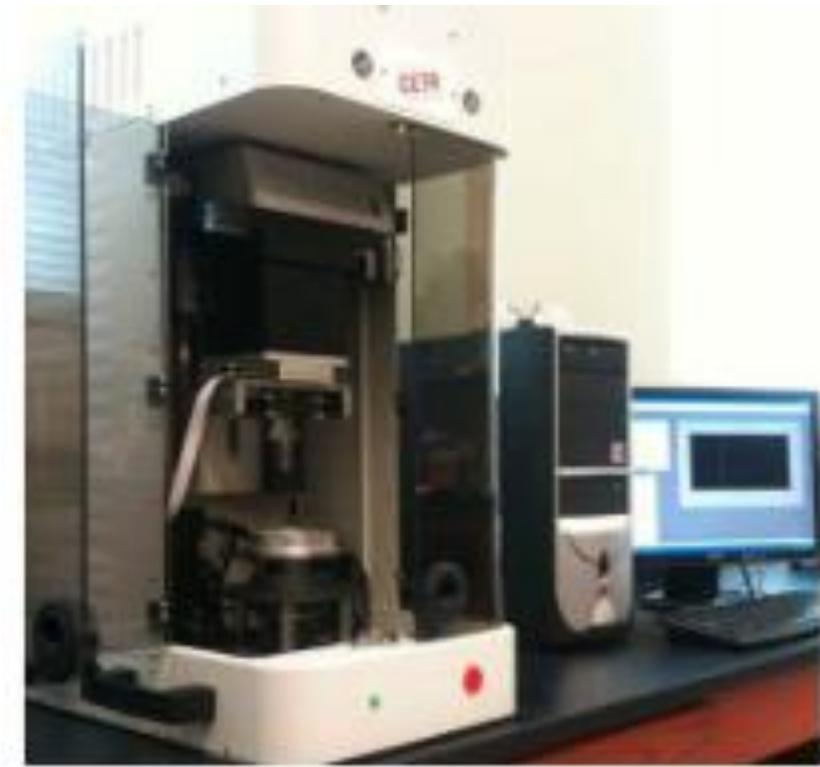
Figure 7. UMT-3 tribometer
