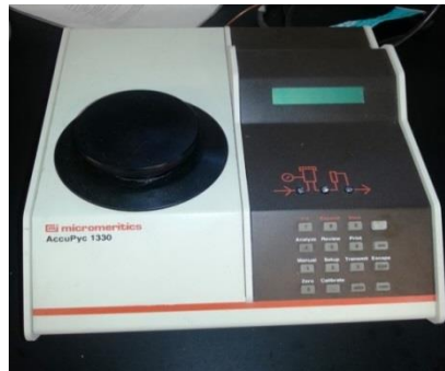
Figure 3.7 AccuPyc II 1330 Pycnometer to measure the volume of biomass
