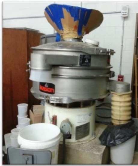
Figure 3.3 Vibratory sieve shaker used for separating soil particles (fine)
