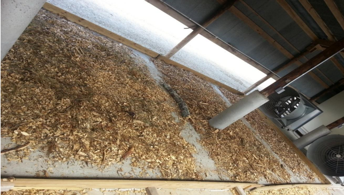
Figure 3.1 Air drying of residual pinewood, whole pinewood and sweetgum
