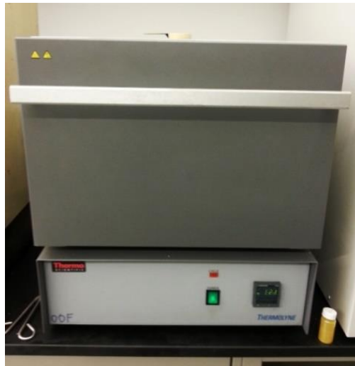
Figure 3.10 Thermo scientific muffle furnace to calculate ash content
