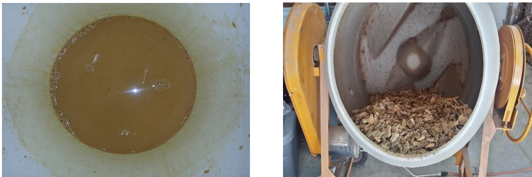
Figure 3.2 Soil and water mixture (left); Coating in mixer (right)
