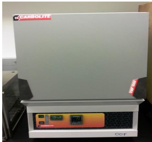
Figure 3.11 Carbolite muffle furnace to calculate volatile matter
