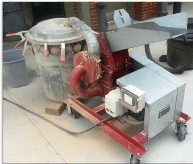
Figure 3.5 Hammer mill used for separation of soil particles from woodchips
