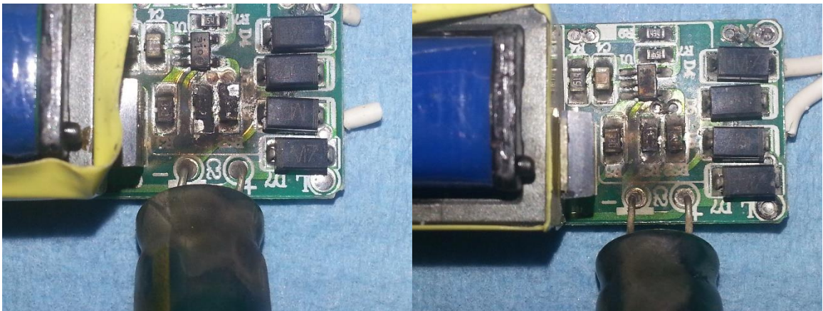
Figure 126: Failure Modes of CHWW 6 (Left) and CHWW 8 (Right) – Catastrophic Degradation of Surface Mount Components and the Aluminum Electrolytic Capacitor.
