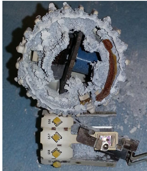
Figure 130: Failure Mode of CWW 3 (Top-Left), CWW 7 (Top-Right) and CWW 9 (Bottom) –Degradation of the Aluminum Heatsink Due to the Exposure to Moisture.
