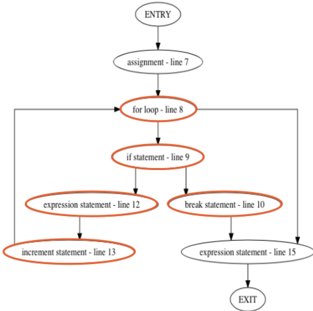
Figure 3.11: Control Flow Graph for Program in Figure 3.10
