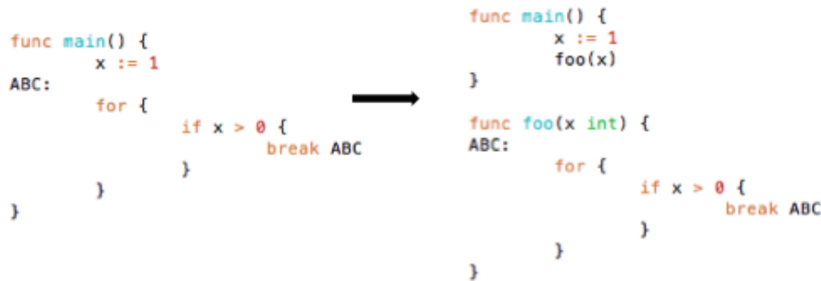
Figure 3.9: Extract Function Refactoring on a labeled branch statement break
