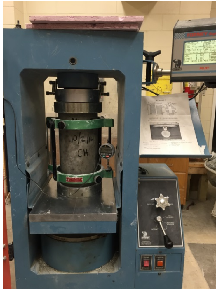
Figure 3-27: Modulus of elasticity testing
