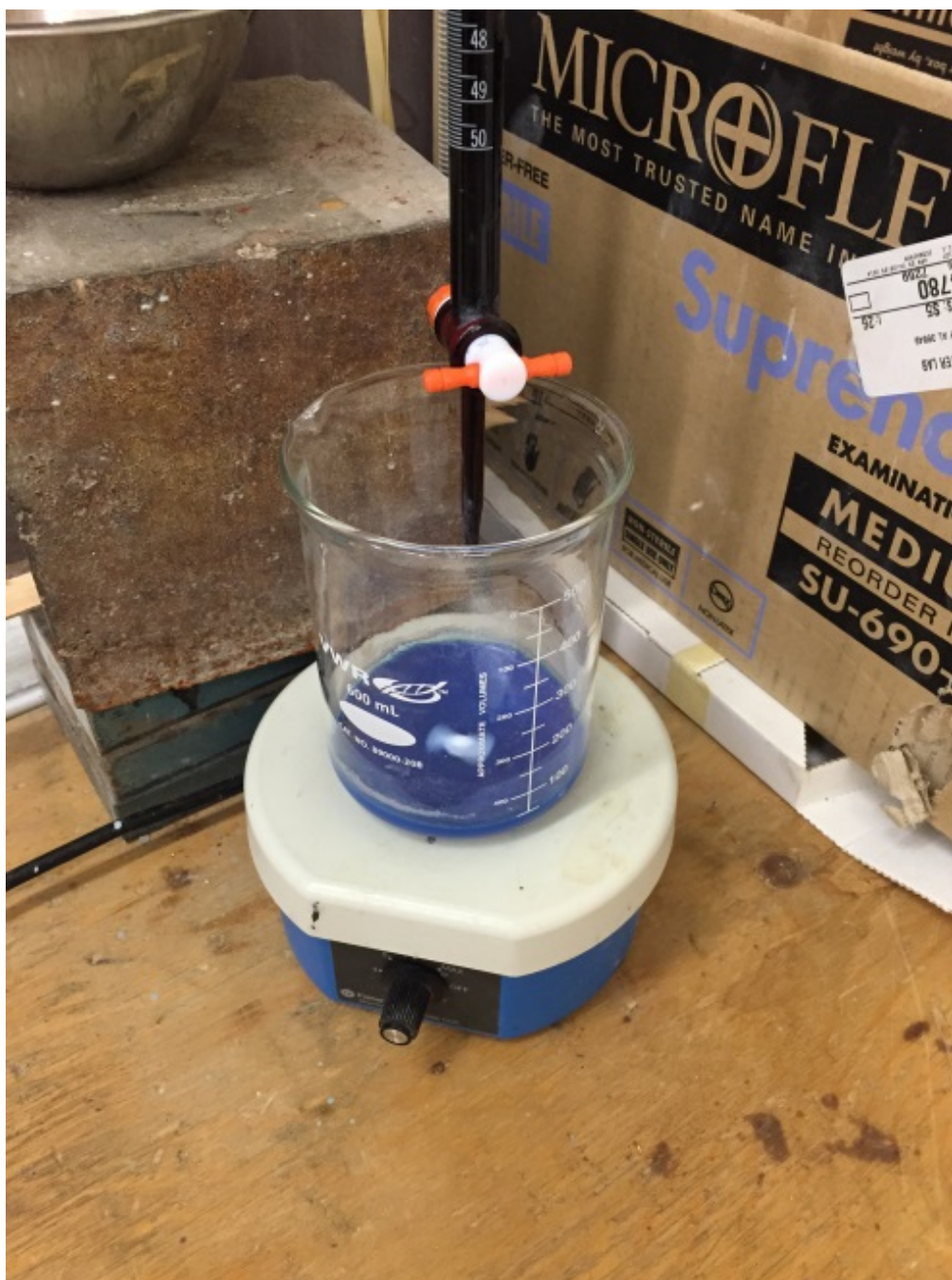
Figure 3-35: Titrating methylene blue solution into slurry
