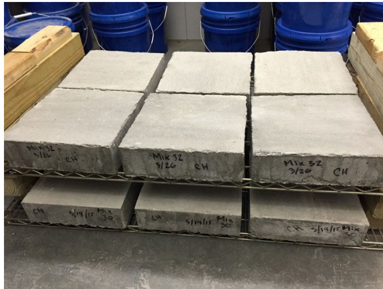
Figure 3-34: Abrasion specimens air cured in laboratory
