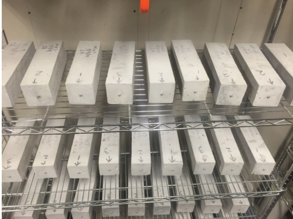
Figure 3-29: Drying shrinkage prisms stored in drying room
