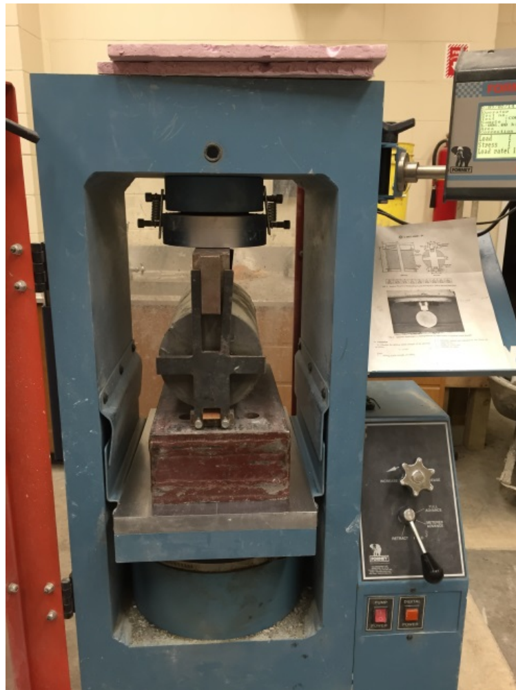
Figure 3-25: Splitting tensile testing arrangement
