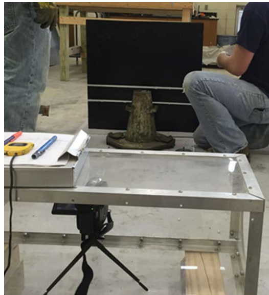
Figure 3-19: Modified slump test setup
