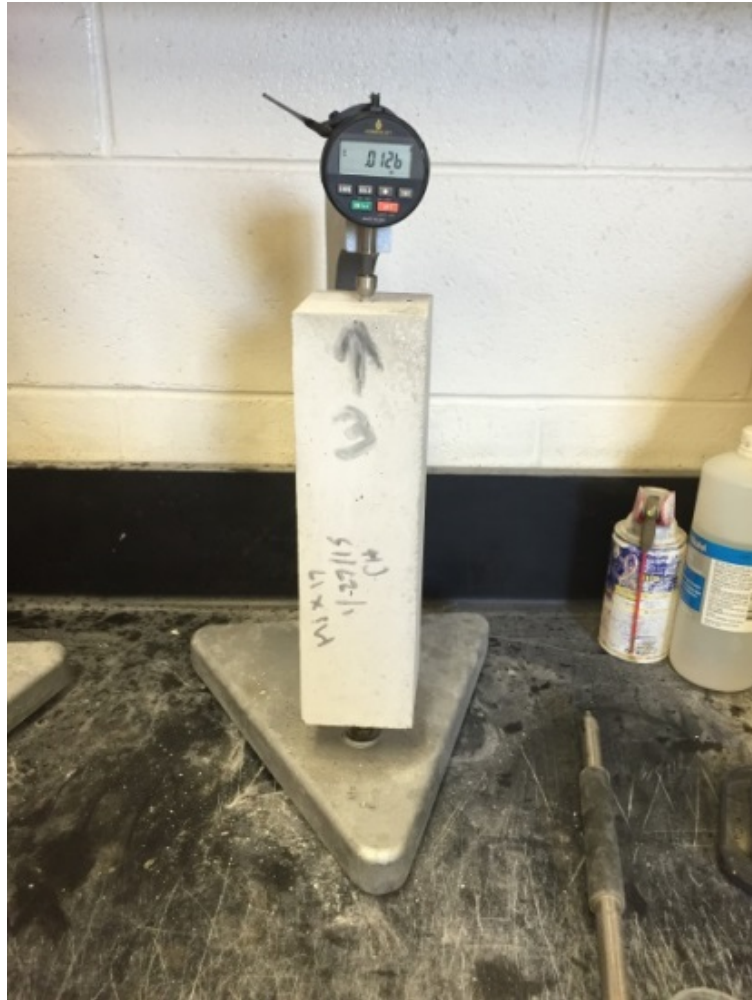
Figure 3-28: Shrinkage prism loaded into comparator
