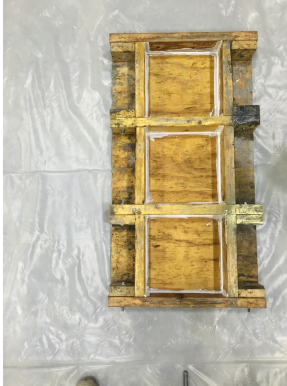
Figure 3-33: Abrasion testing formwork
