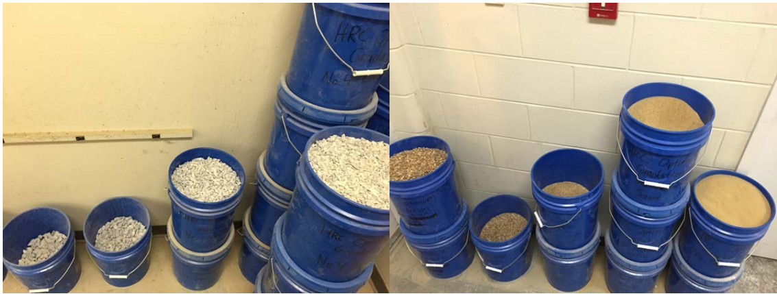
Figure 3-14: Dolomitic limestone and river gravel aggregates separated by sieve size
