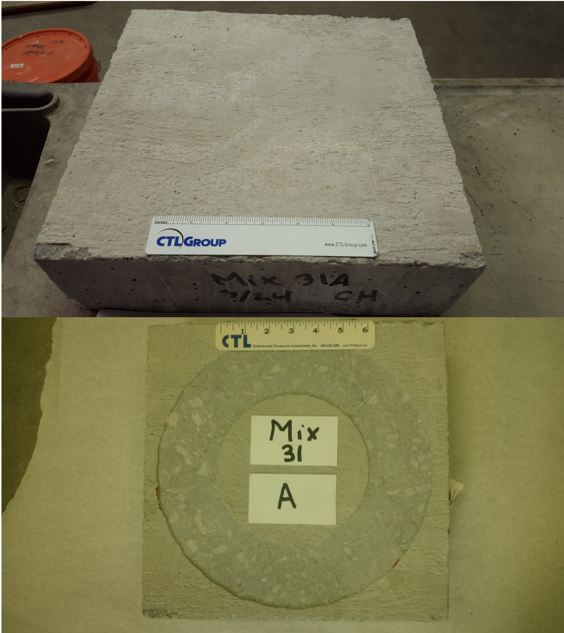
Figure D-2: Before (top) and after (bottom) pictures for dolomitic limestone 5% dust-of-fracture mineral filler
