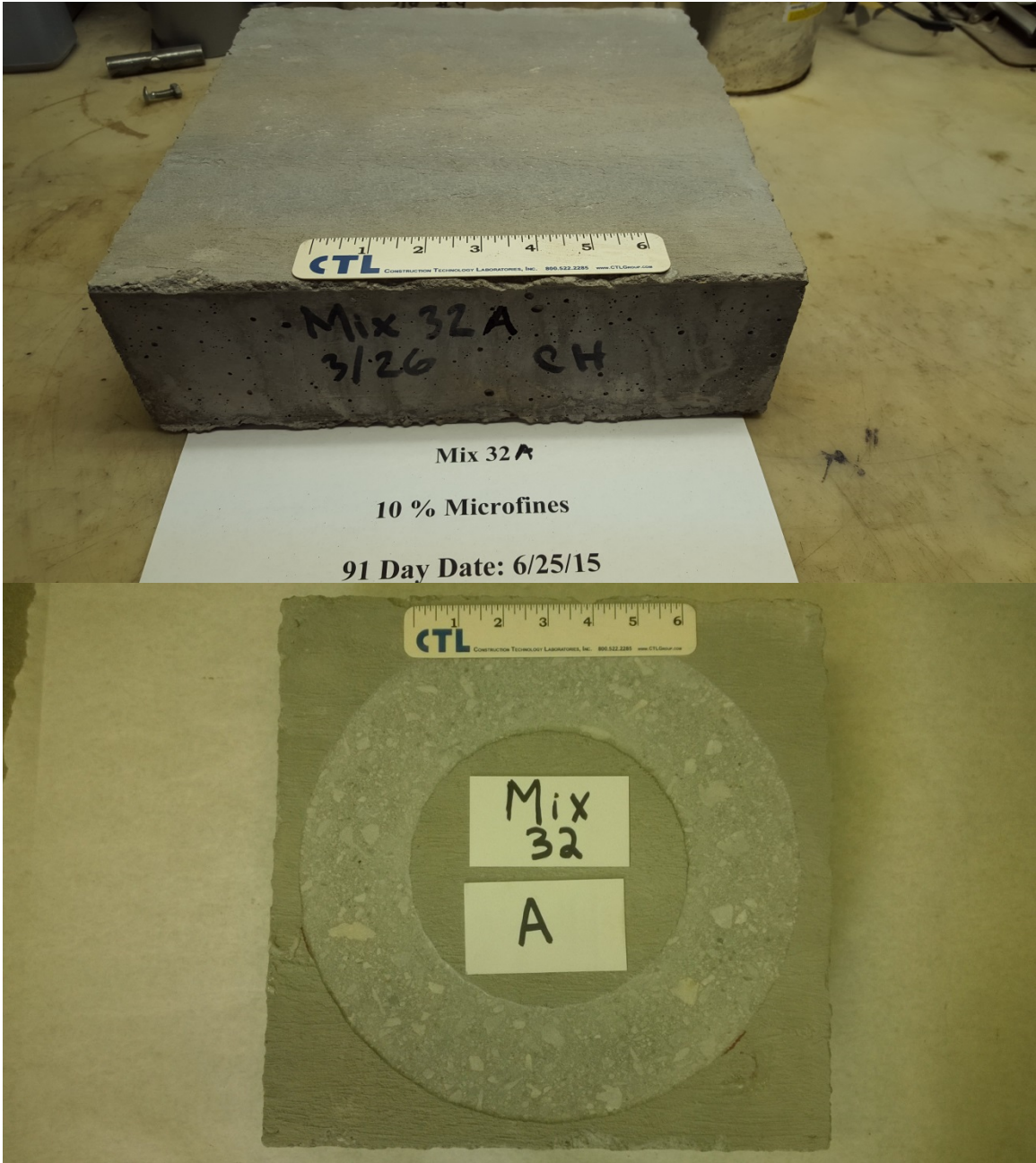
Figure D-3: Before (top) and after (bottom) pictures for dolomitic limestone 10% dust-of-fracture mineral filler
