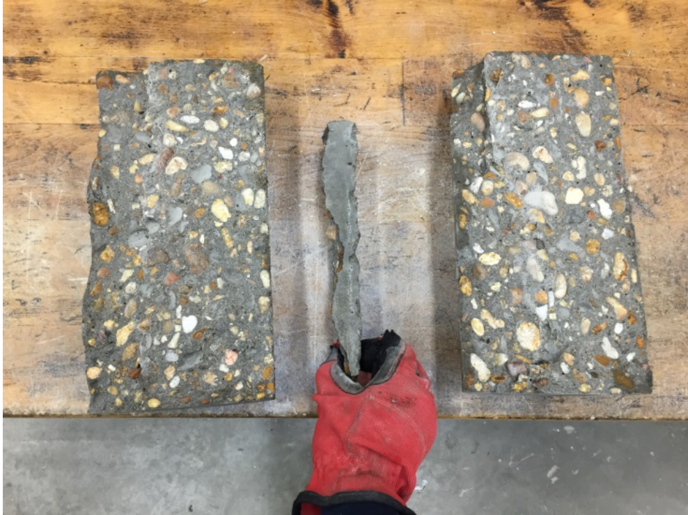
Figure 3-26: Splitting tensile fracture
