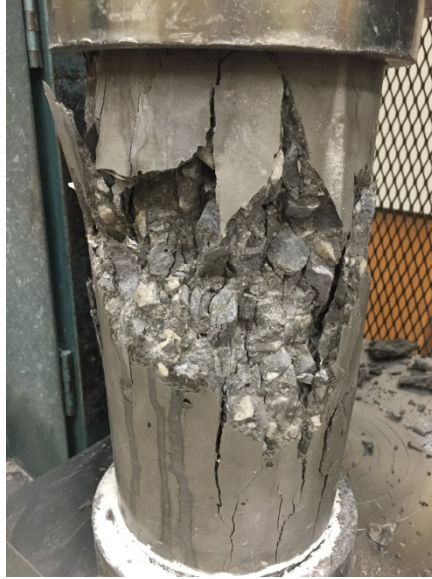
Figure 3-24: Compression testing fracture pattern
