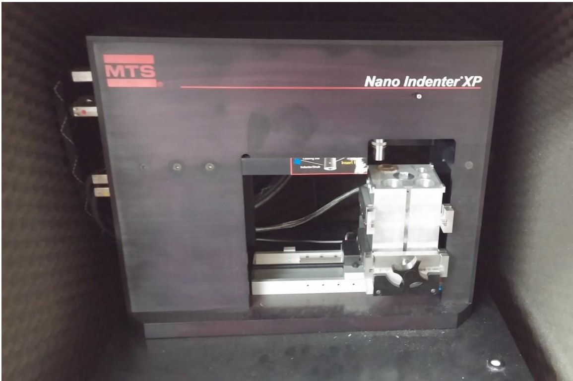
Figure 15. MTS Nanoindenter XP at Auburn University, Materials Engineering Department, 2015.
