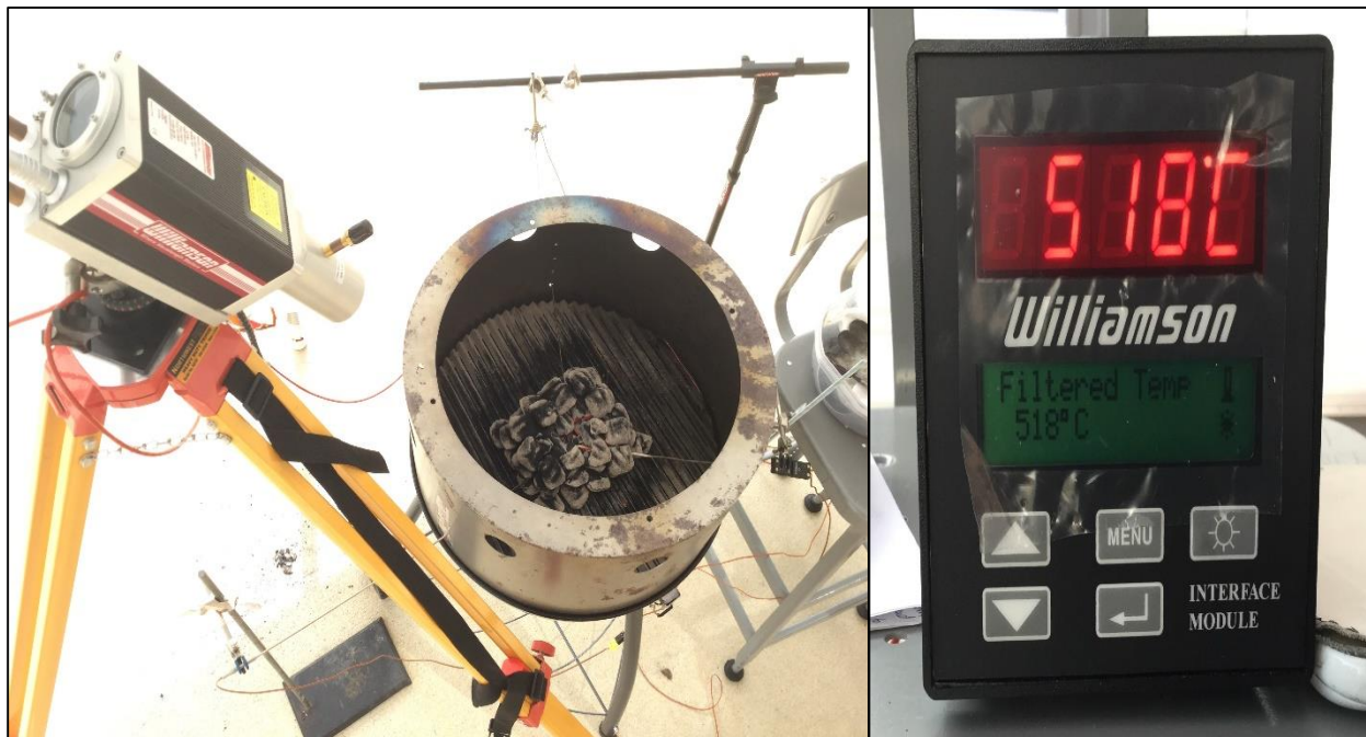
Figure 3. 1 Williamson SW Pyrometer (on the left) and Interface module (on the right)
