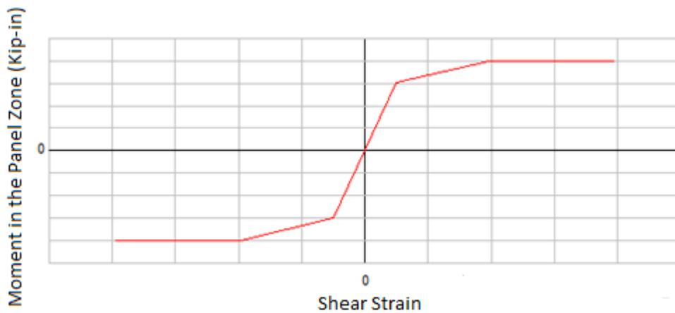
**Figure 3-31: Relationship between Moment and Shear Strain in the Panel Zone**
