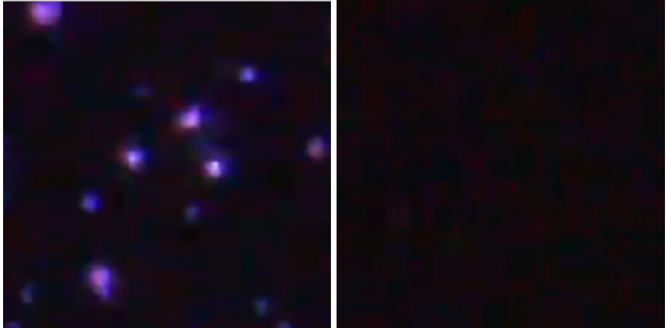
Figure 4.6 Images from an optical microscope equipped with a dark field condenser of JNPs with a PEG functionalized hemisphere (image enlargement using digital zoom has been applied). In the left side image, no filter is being applied; on the right side image, a fluorescent filter is applied to limit the incoming light to between 470 nm and 525 nm.
