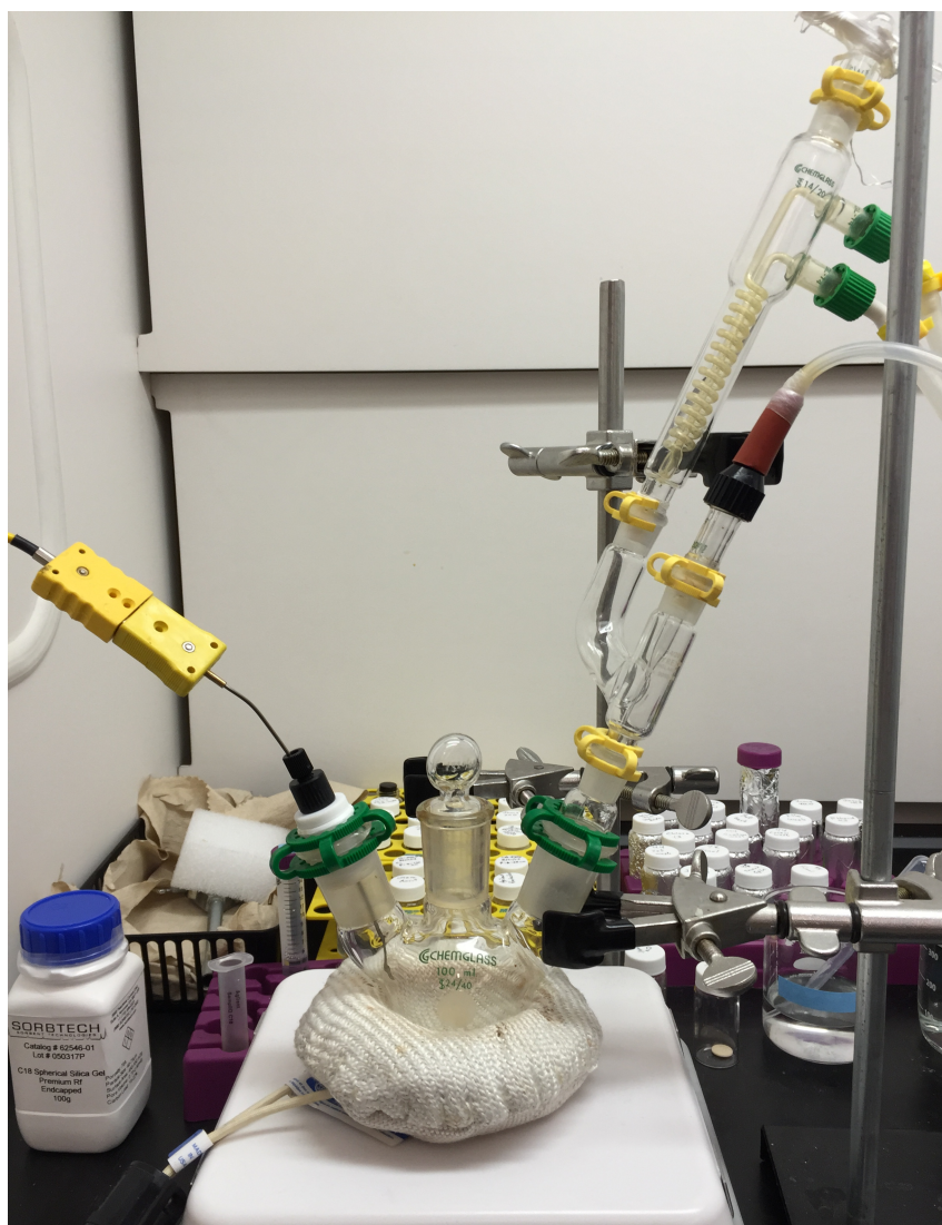
Figure 2.1 Setup of reaction vessel for synthesizing O-MNPs
