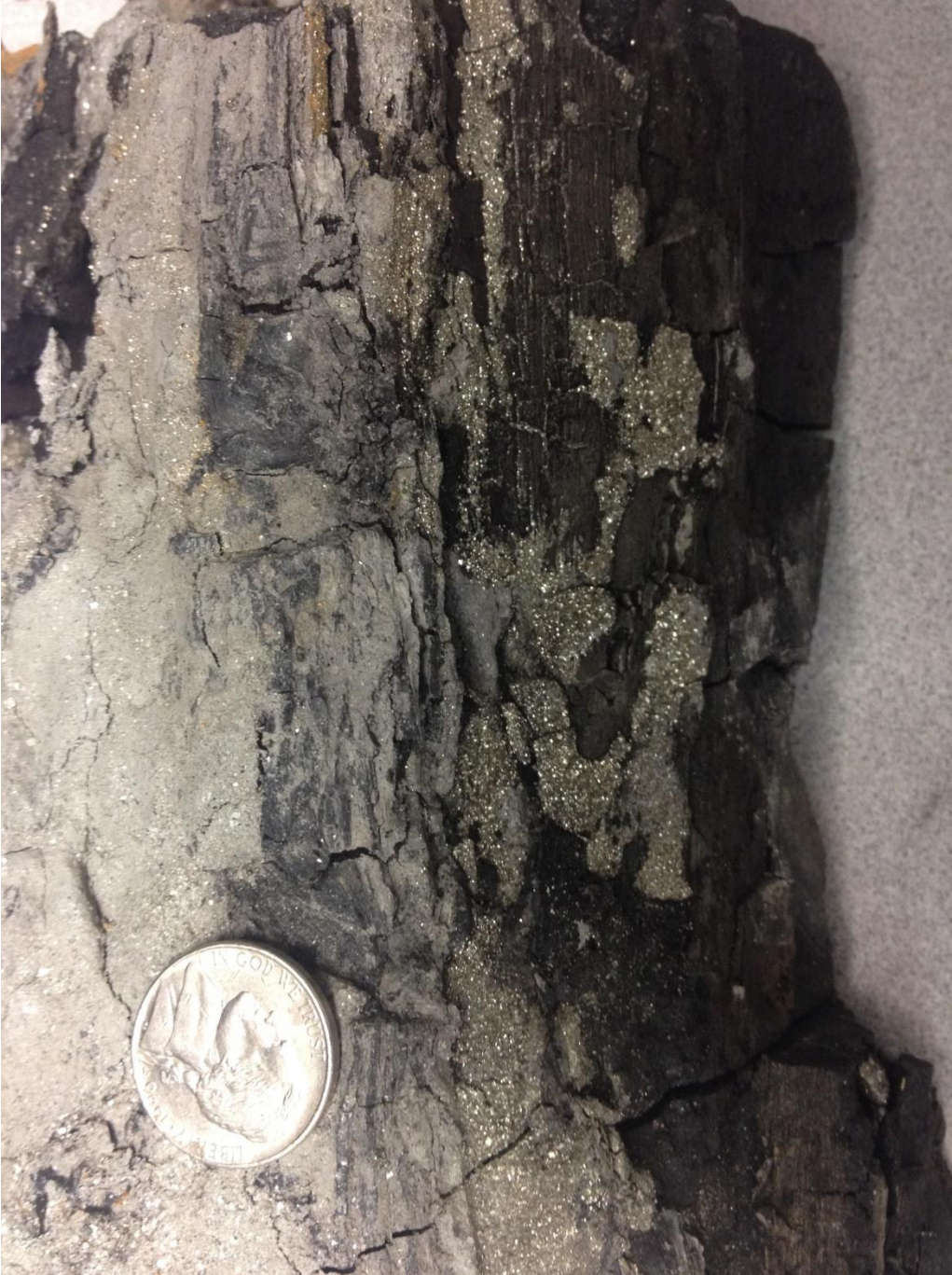
Figure 14. Biogenic pyrite sample from Macon County, AL submitted to ACME Labs Inc. for aqua regia digestion and ICP-MS testing.
