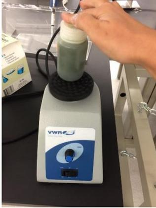
**Figure 3.14: Mixing of the biomass samples by VWR Analog Vortex Mixer.**
