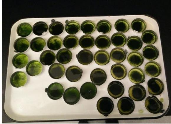
**Figure 3.15: Algal samples before putting in the conventional oven at 105°C.**
