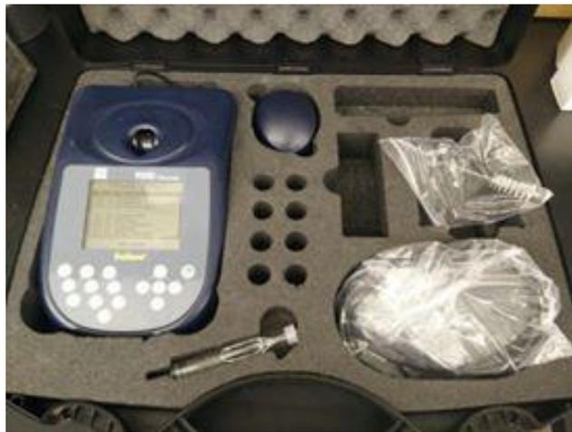
**Figure 3.20: YSI 9500 Photometer.**
