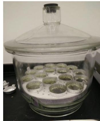
**Figure 3.17: Dried algal samples in the desiccator.**
