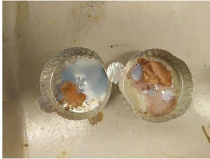
**Figure 3.18: Algae samples after removing from the muffle furnace.**
