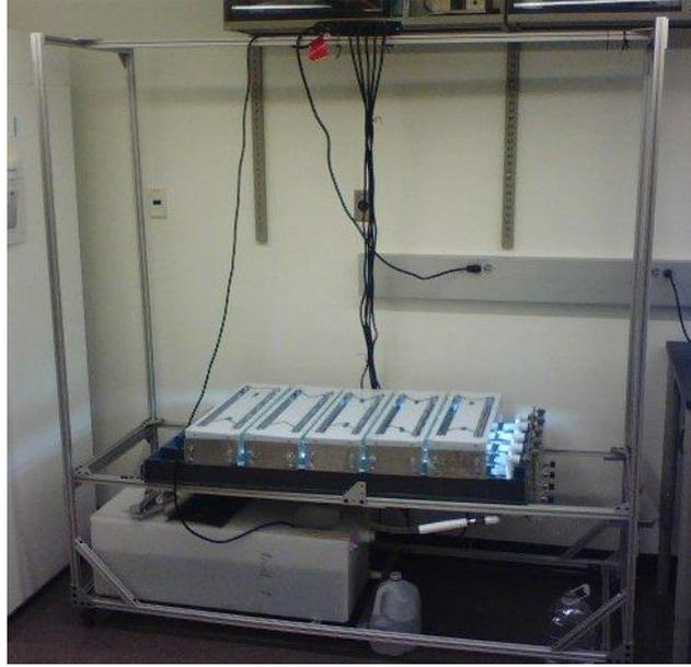
**Figure 3.1: Flow lane incubator and frame assembly.**
