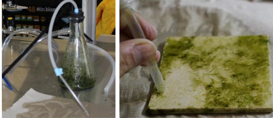
**Figure 3.11: Vacuum harvesting apparatus (left) and vacuuming process (right).**
