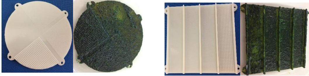
**Figure 2.7: Circular and rectangular tiles before and after biofilm colonization in an ATS.**
