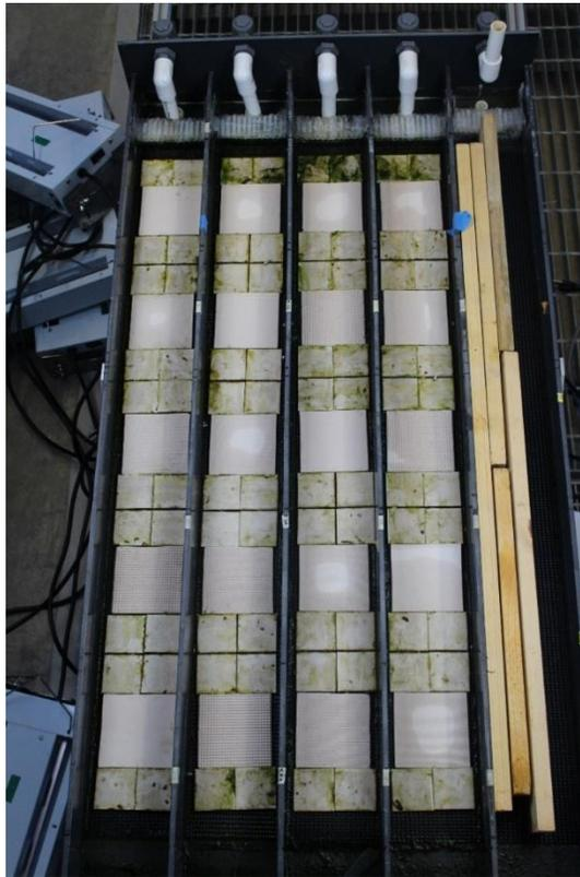
**Figure 3.7: Placement of tiles on the flow lane photo incubator.**
