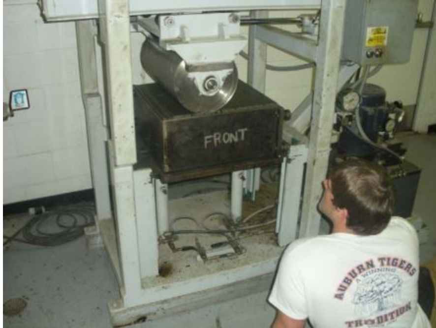
Figure 31 – Kneading Compactor for 20 x20 inch slabs (Tran, 2012)
