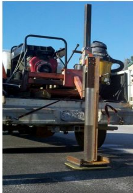
Figure 22 – NCAT Truck-Mounted Field Permeameter
