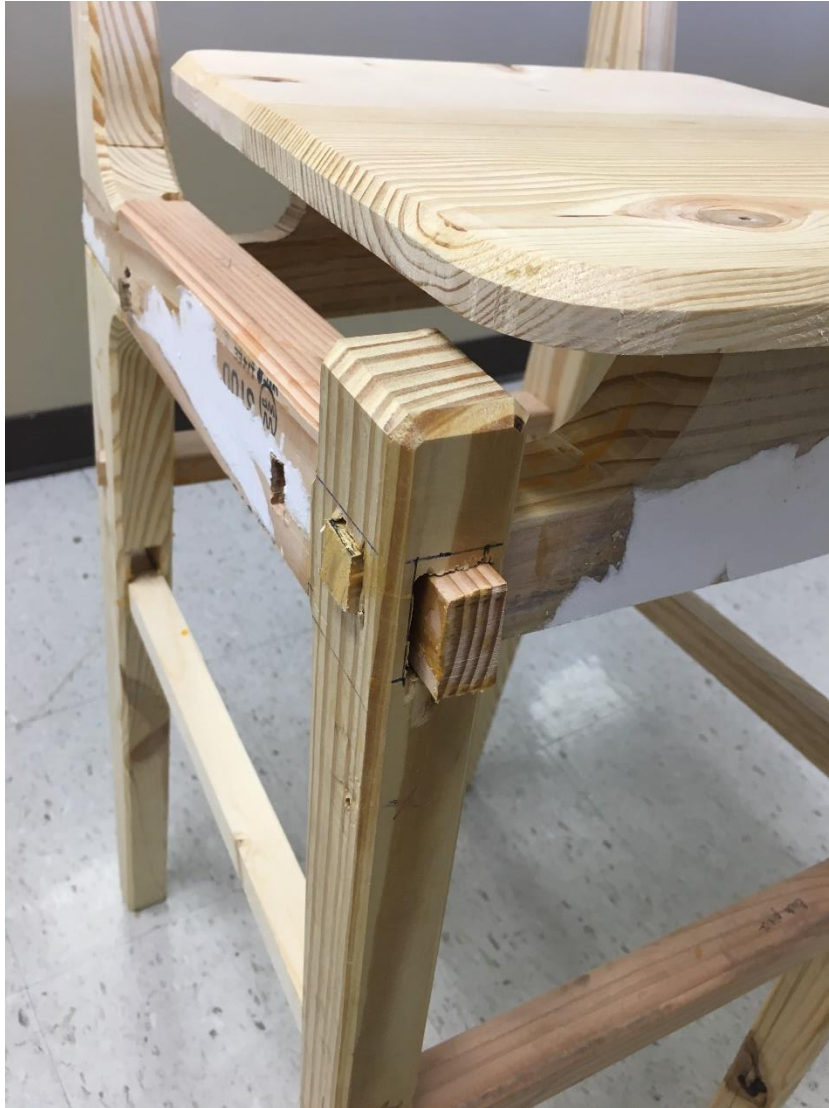
Figure 49, Front piece tenon joint detail.
