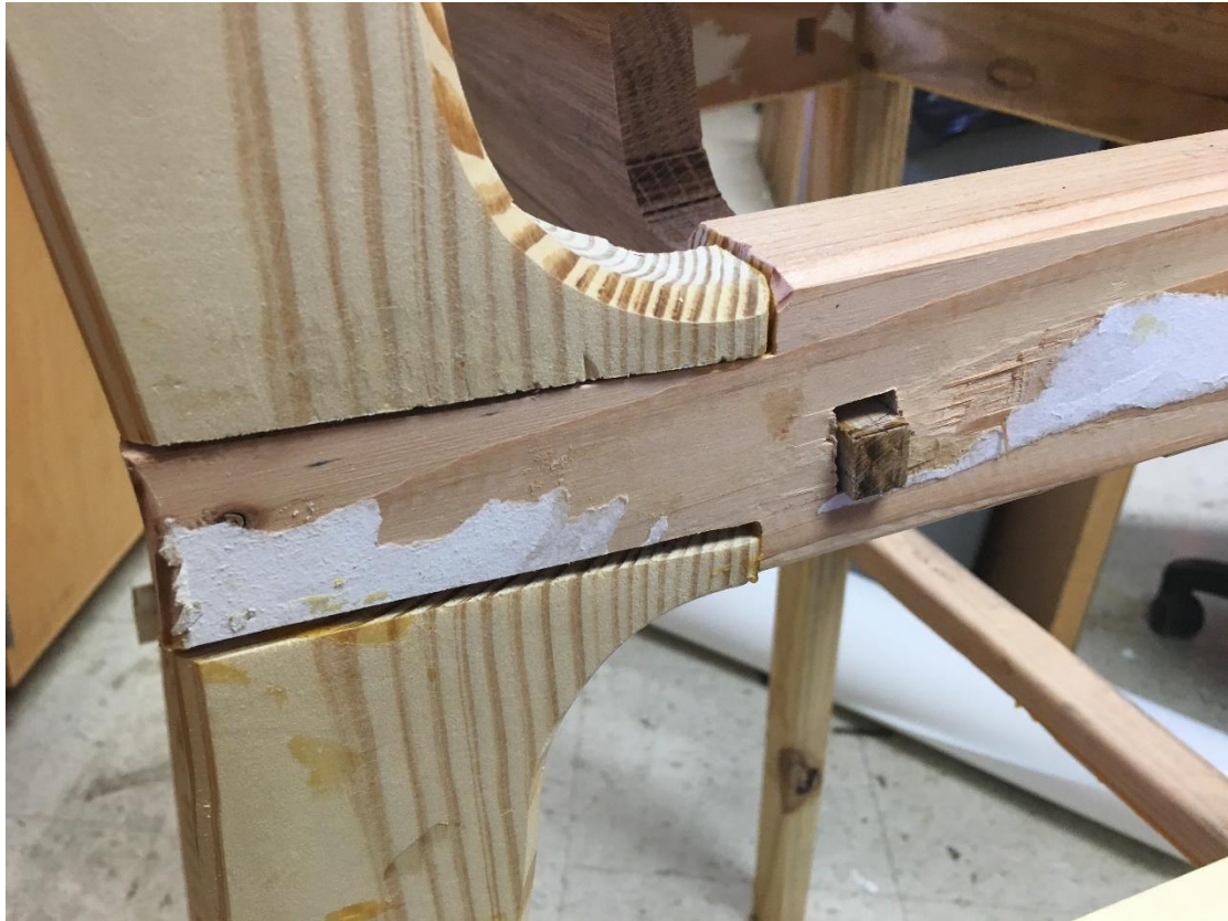
Figure 48, Testing model, tenon joint detail
