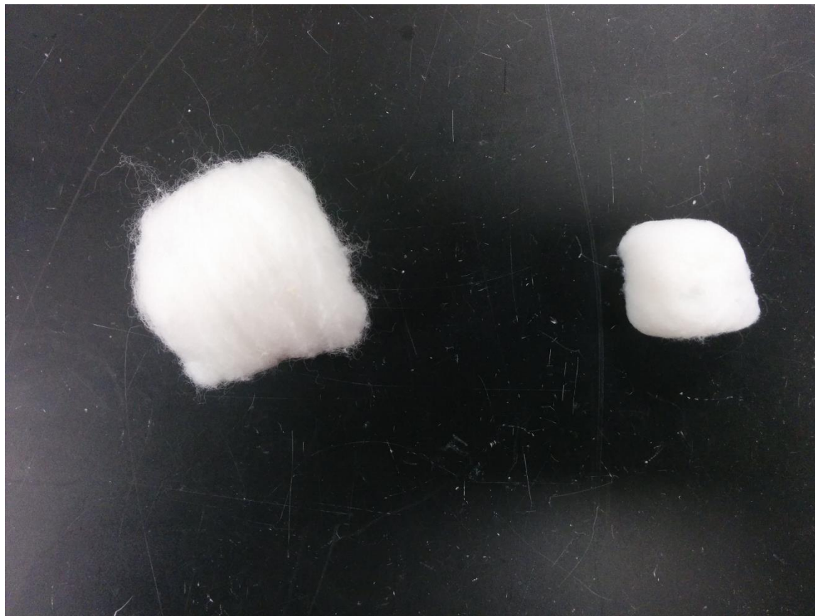
Figure 5.2. Cellulose cotton ball before treatment (left) and silica support following cellulose removal (right).
