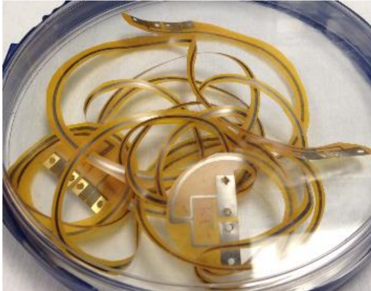
Figure 2.30: One meter long microstrip transmission line on Kapton in its final form.
