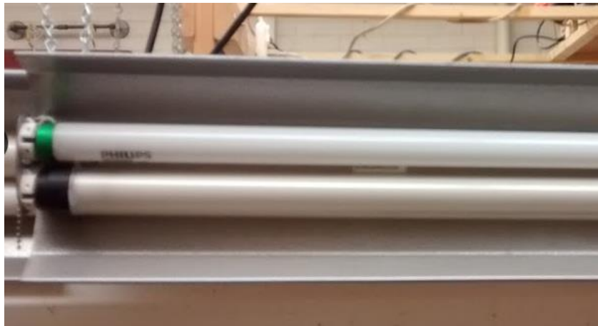
Figure 3.4. View of a light fixture used to house the Phillips cool white lamp (top) and (filtered) Heliovite UV lamp (bottom).
