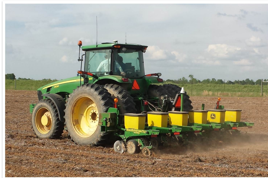
Figure 3.1: Image of the 6-row John Deere planter equipped with MaxEmerge Plus Row-Units used in this research.
