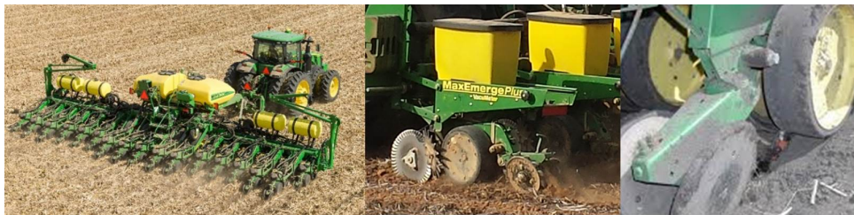
Figure 1.2: Modern row-crop planters are constituted of individual row-units designed to place seeds in the ground at a proper and predetermined depth. Seeding depth is controlled through the use of two gauge-wheels mounted on individual planter row-unit.
