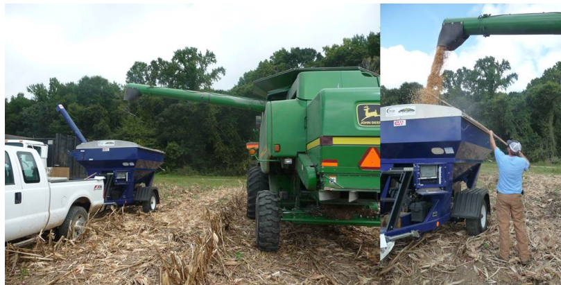
Figure 3.19: Weight wagon used to calibrate yield monitor data at every plot, and collection of grain sample to adjust final yields at 15.5% moisture content.
