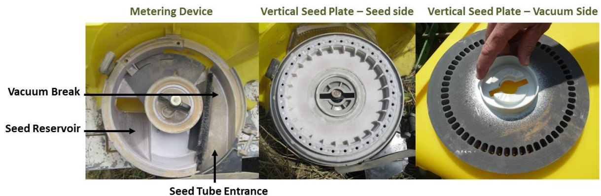
Figure 2.2: Illustration of the vacuum-disk metering system.
