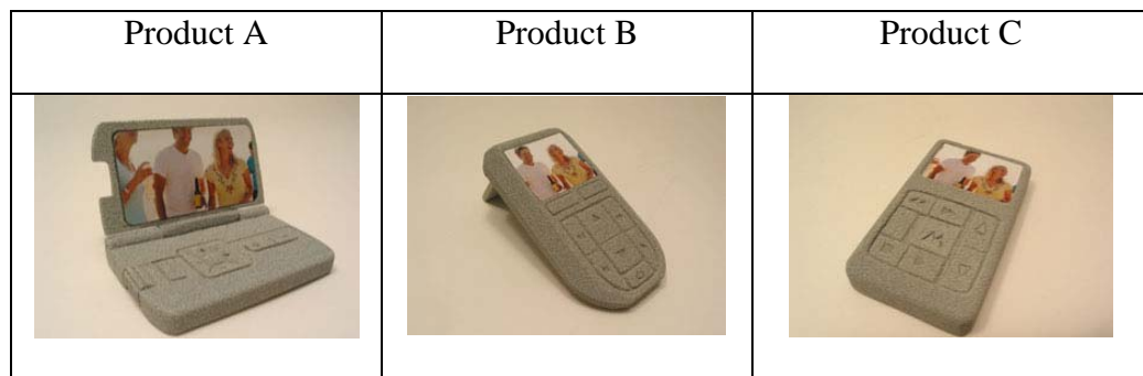
Figure 4.3 - Session 3 Pre-Prototypes made of urethane foam
