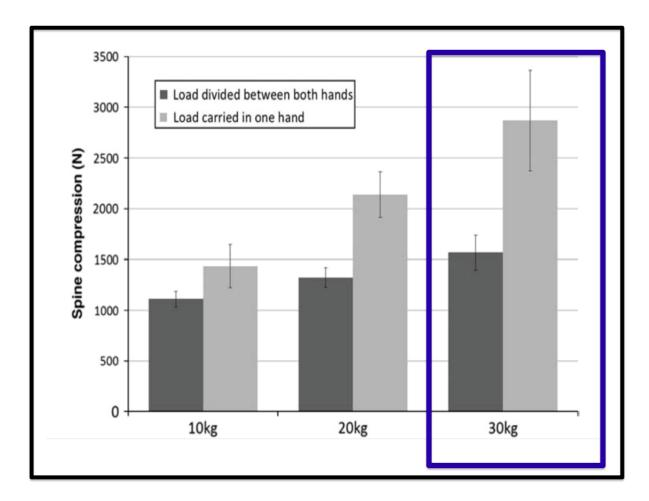
Figure 2.5: Difference in spinal compression when load is divided between both hands vs. being lifted by one hand. [McGill et al., 2013]
