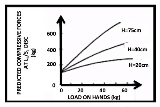
Figure 2.3: Predictive back compressive forces acting on the L5/S1 discPredictive back compressive forces acting on the L5/S1 disc. (Adapted from Chaffing, 1975). [NIOSH, 1981]
