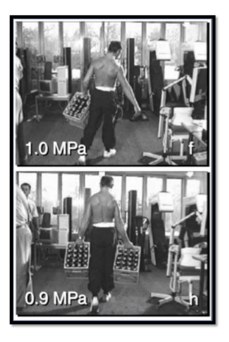
Figure 2.4: Differences in back compressive force when subject performs one-hand and two-hand lifts. [Wilke et al., 2001]
