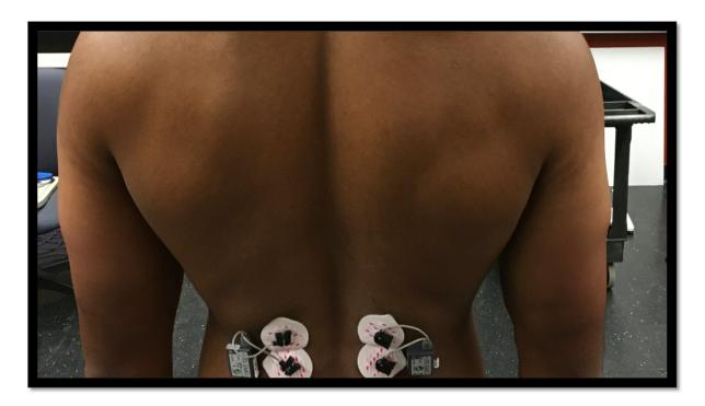
Figure 3.5: Example of Sensors and Electrodes Placed Near the Erector Spinae Muscles
