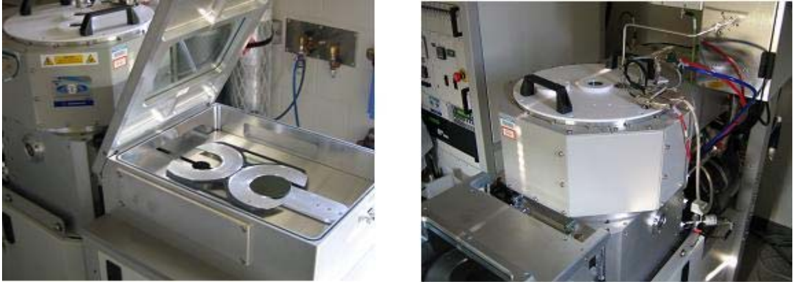
Figure 2.6: STS Multiplex ICP used to etch silicon.
