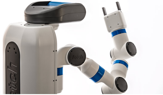
(b) Fetch's robot hand for order retrieval
