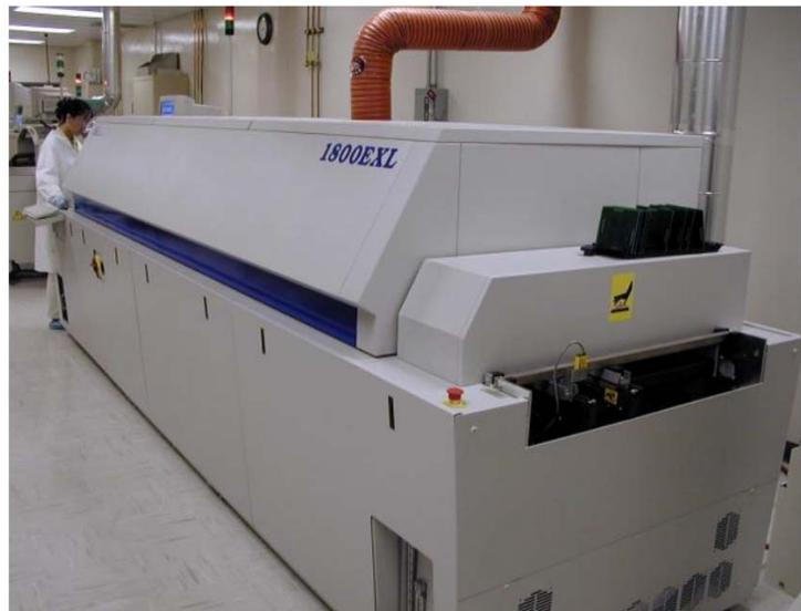
Figure 2.4 - Heller 1800EXL Reflow Oven
