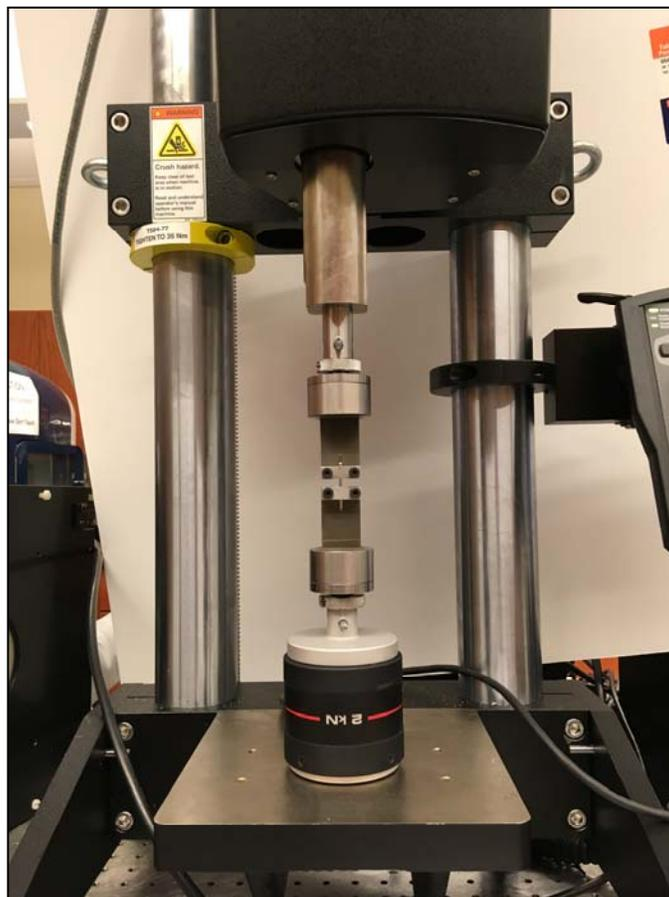
Figure 7.6 - Instron 5948 Microtester with the Fixtures
