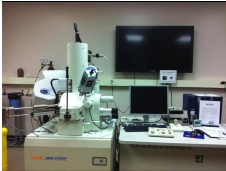
Figure 2.15 - JEOL JSM-7000F Field Emission SEM
