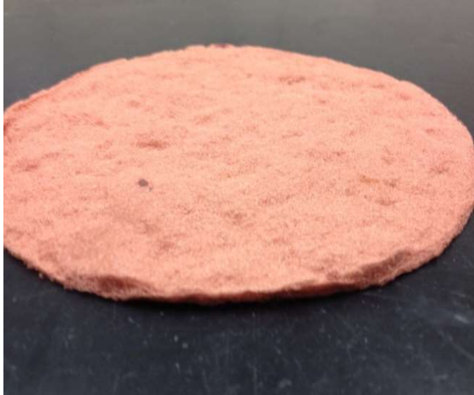
Figure 2. Example of a copper MFEC sheet after sintering, prior to catalyst entrapment.
