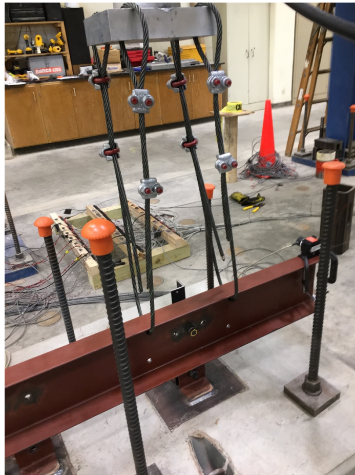
Figure 3-6: Experimental Setup for Application of Out-of-Plane Force
