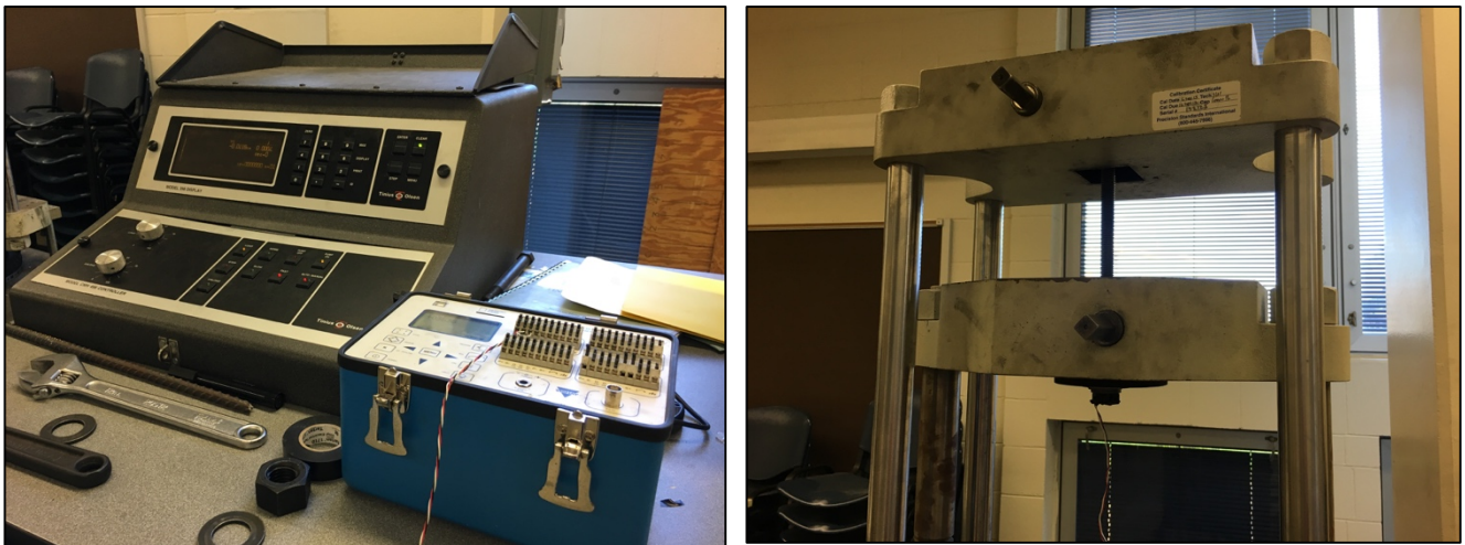
Figure 3-8: Experimental Setup for Bolt Calibration
