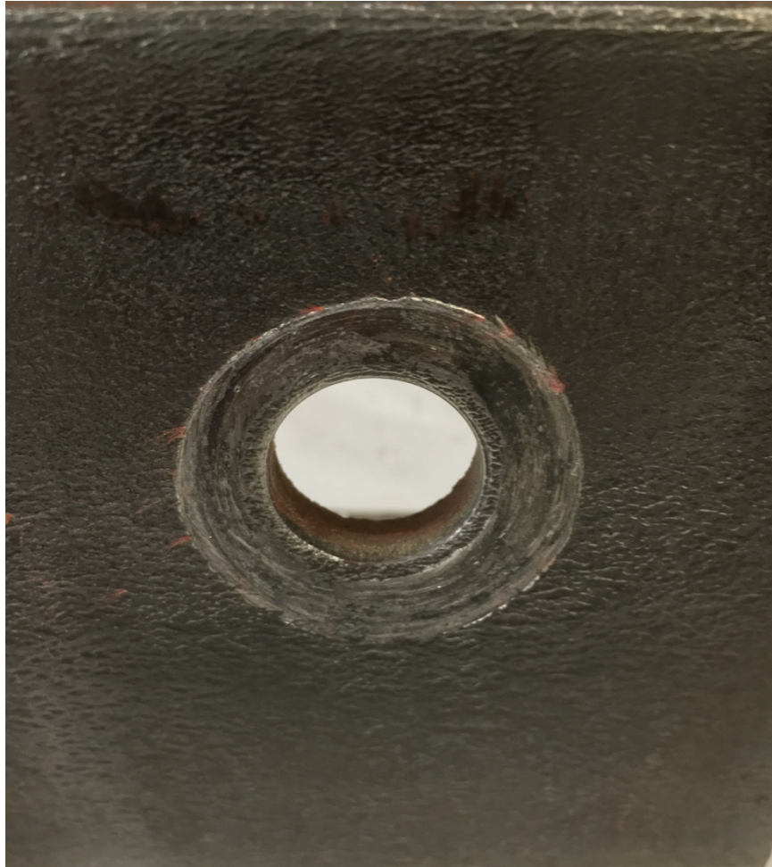
Figure 4-17: Damage on Interior Face of Angle after Three 100-Cycle Tests
