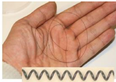
Figure 35 - Coil-spring greatly increases strain [59] [114] (device #1)
