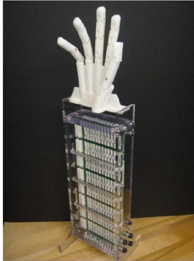
Figure 53 - Prosthetic hand with clever open-loop control system [136] [140]
