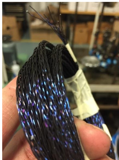
Figure 71 - Braided NiTi rope offers improved flexibility, much lower cost, and much faster heat transfer than a solid rod of equal weight
