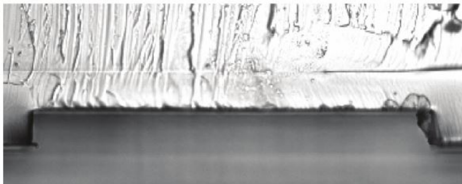
Figure 5.3: Fluidic current mirror ROI channel cross-sections ROI region cross-section for the autoregulator current mirror (38 \mu\text{m} high and 477 \mu\text{m} wide).
