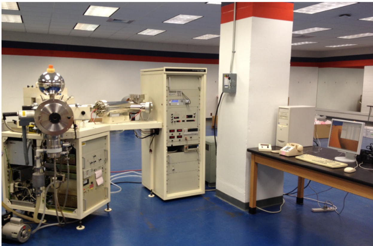
Fig. 14. Thermal ionization mass spectrometer (TIMS, Finnigan MAT 262) at the Trace Metal Isotope Laboratory at Auburn University.
