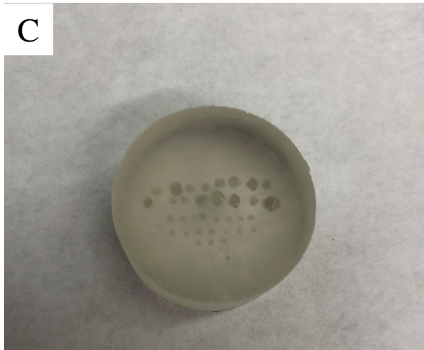
Fig. 15. A) Close up of quartz grains placed on double sided- sticky tape. B) Teflon mold with quartz grains in epoxy. C) Final polished grain mount.
