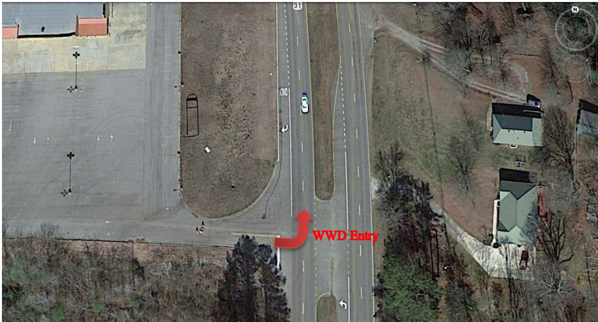
FIGURE 15 Unsignalized Intersection of US Highway 31 (Divided Highway) and IGA store parking lot driveway (Crossroad) in AL
