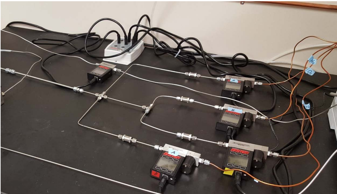
Figure 8: Gas mixing system developed for systemic studies. a) Schematic of mixing system b) Actual mixing system.
