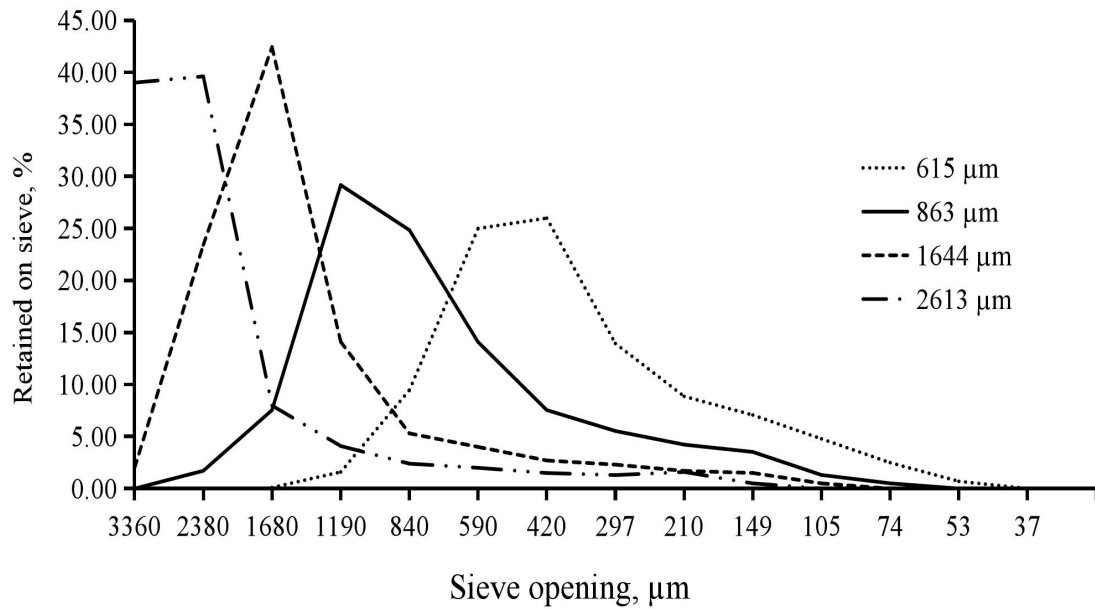
Figure 3.3 In trial 3, the geometric mean diameter by mass ( D_{gw} ) and particle size distribution of corn prior mixing during was determined in the finisher period from 28 to 42 d of age. Ross × Ross 708 male broilers were fed 4 corn particle sizes over the finisher period from 28 to 42 d of age (n=10). Dietary treatments were obtained by grinding whole corn with a roller mill (615, 863, 1,644 and 2,613 µm) and diets were offered in a pelleted form. Common starter and grower diets were fed from 1 to 14 and 14 to 28 d of age, respectively.
