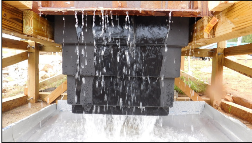
FIGURE 4.21 WQS with water flowing around device.
