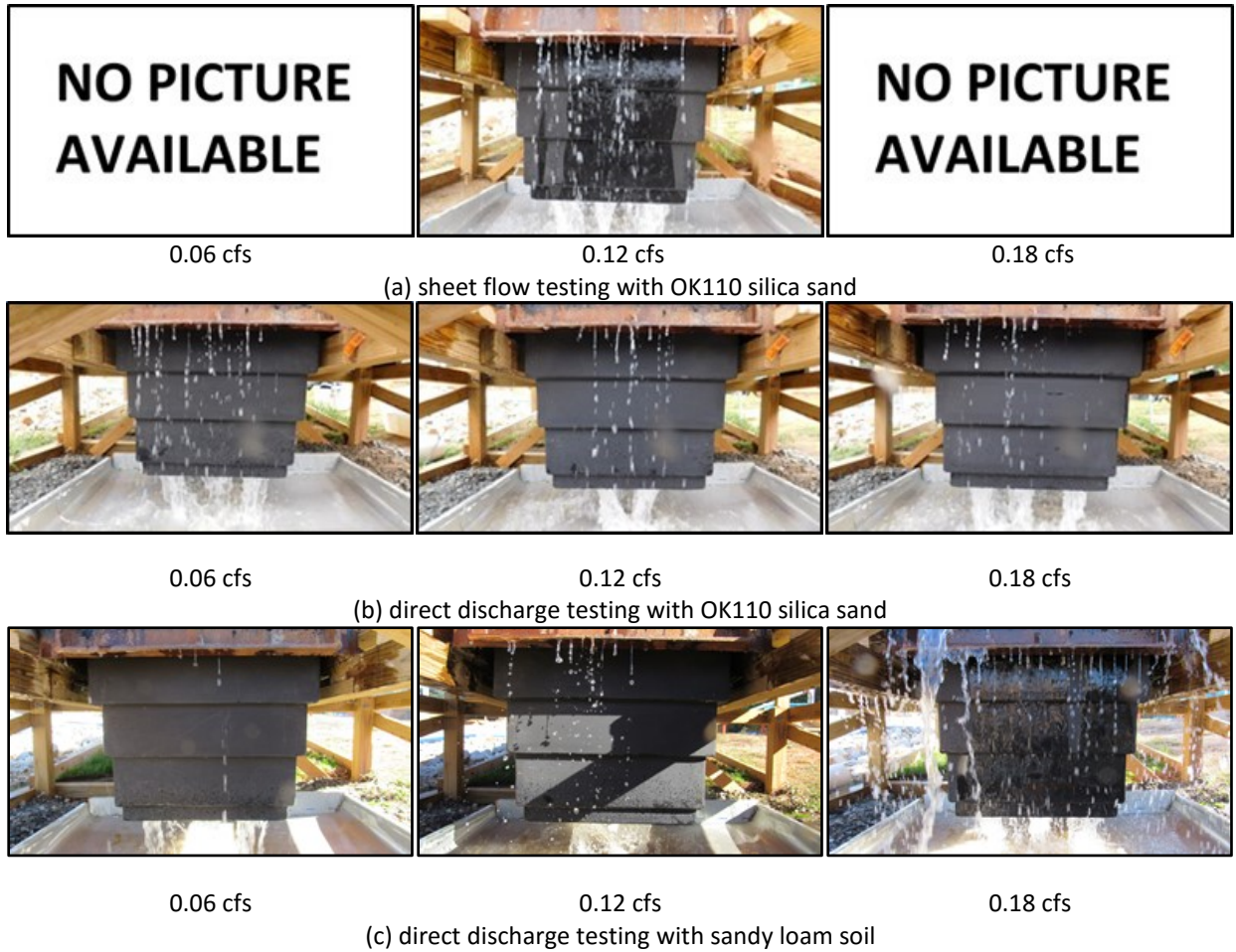
FIGURE 4.20 WQS during testing using various test methods and soil types.
