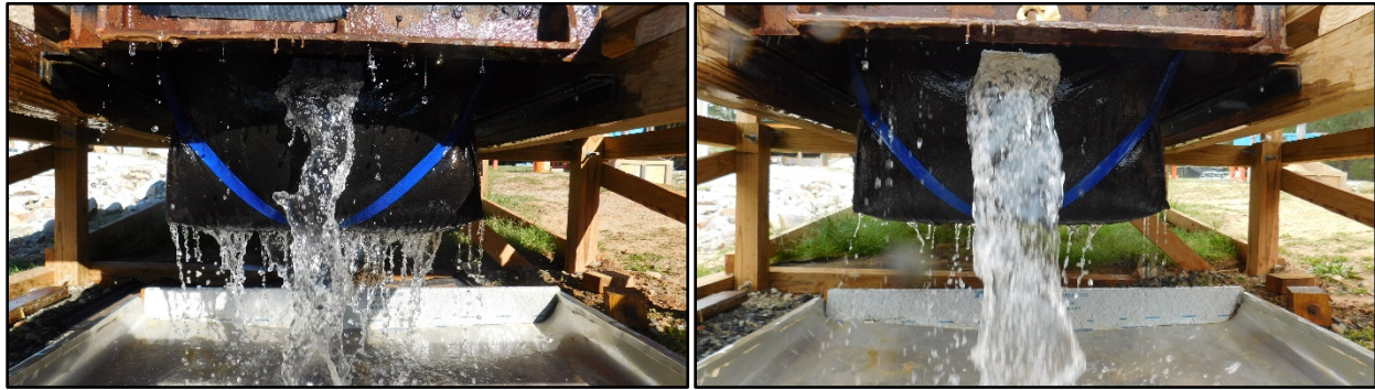
(a) L1 (b) L2 FIGURE 4.28 Gullywasher during longevity testing with sandy loam soil.
