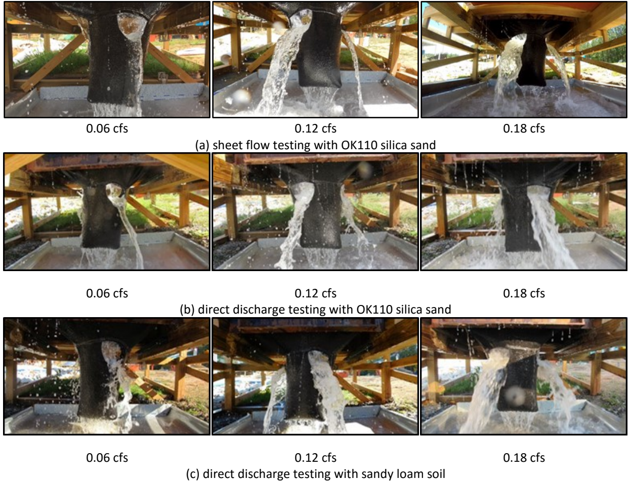
FIGURE 4.16 Storm Sentinel during testing using various test methods and soil types.
