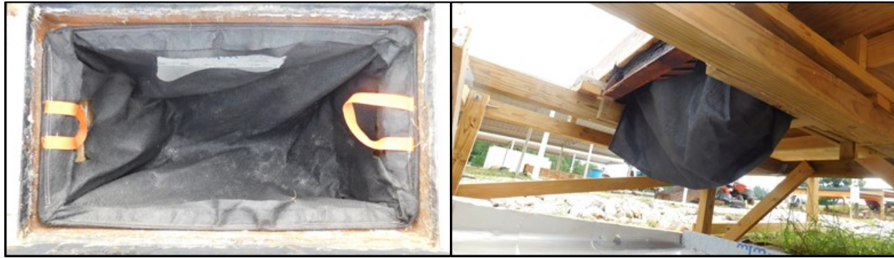
(a) interior of non-proprietary CBI
