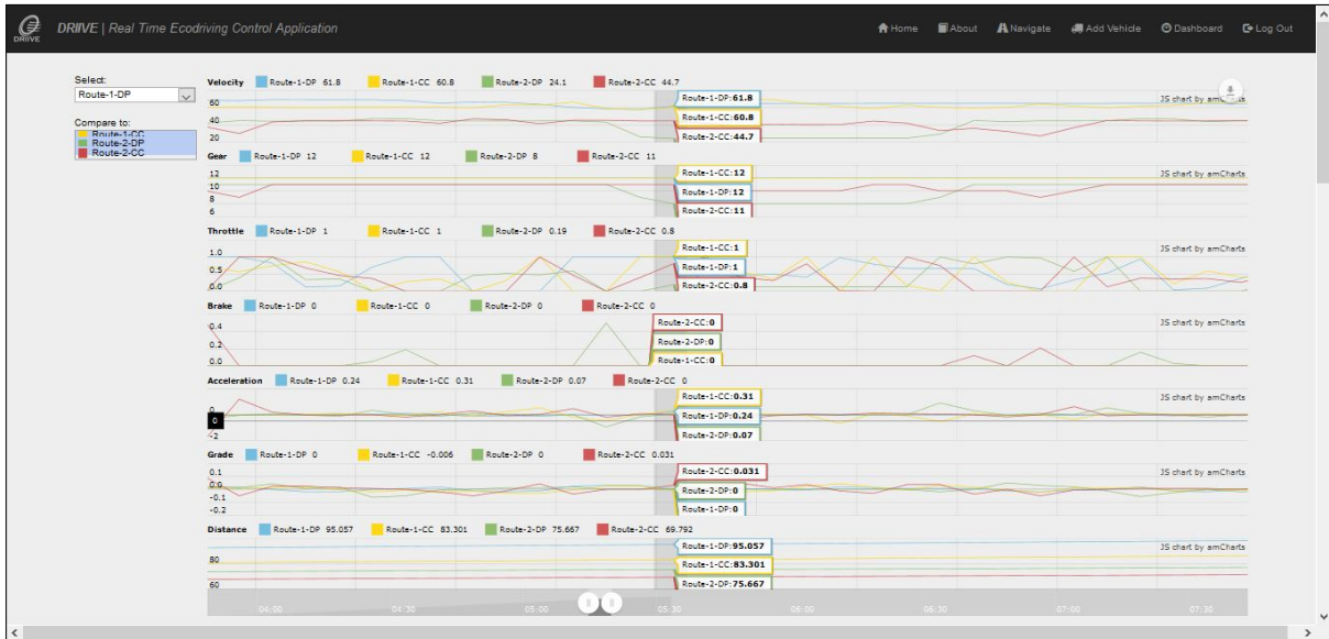
Figure 3.28: A snapshot of the final version of the page "Graphs" page. Once the web application is used for an origin-destination pair, a user can select, from the drop-down menu on the top-left corner of the page, up to six routes to simultaneously compare their performances over time in terms of velocity, gear, throttle, brake, acceleration, road grade, and distance through the course of the trip. When the cursor hovers over one point in time, the exact values of selected routes appear next to the cursor, simultaneously. A button on the top-right corner of this page allows users to download all these data for further analysis. For this figure, two routes are selected by a user.
