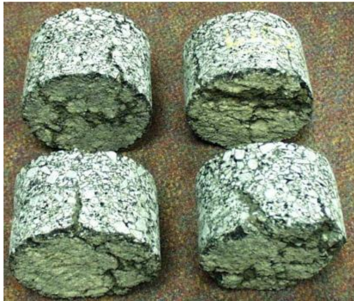
Figure 1. Bottom-up Cracking (Gibson et al., 2012)
