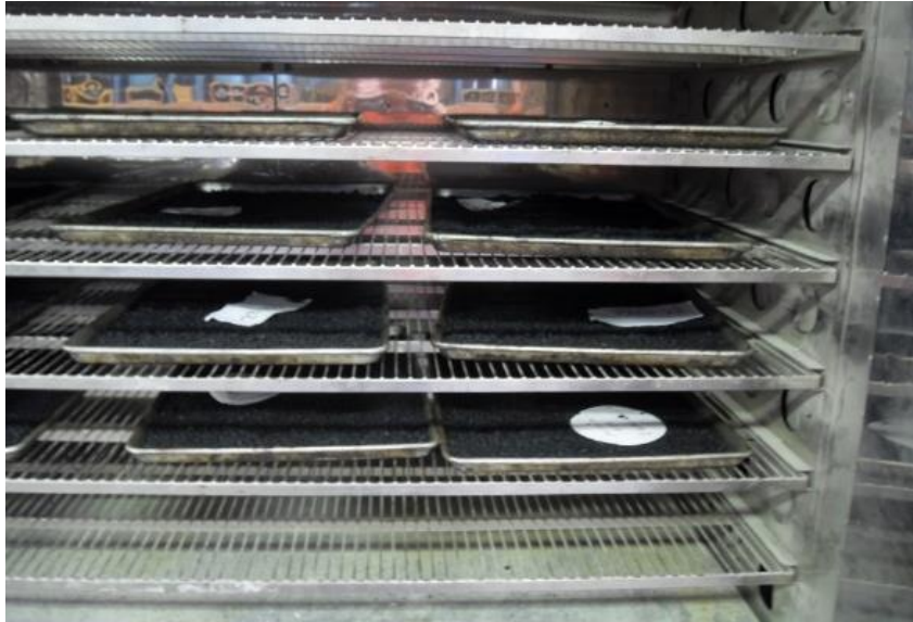
Figure 32. Loose Mix Long-term Aging in Oven
