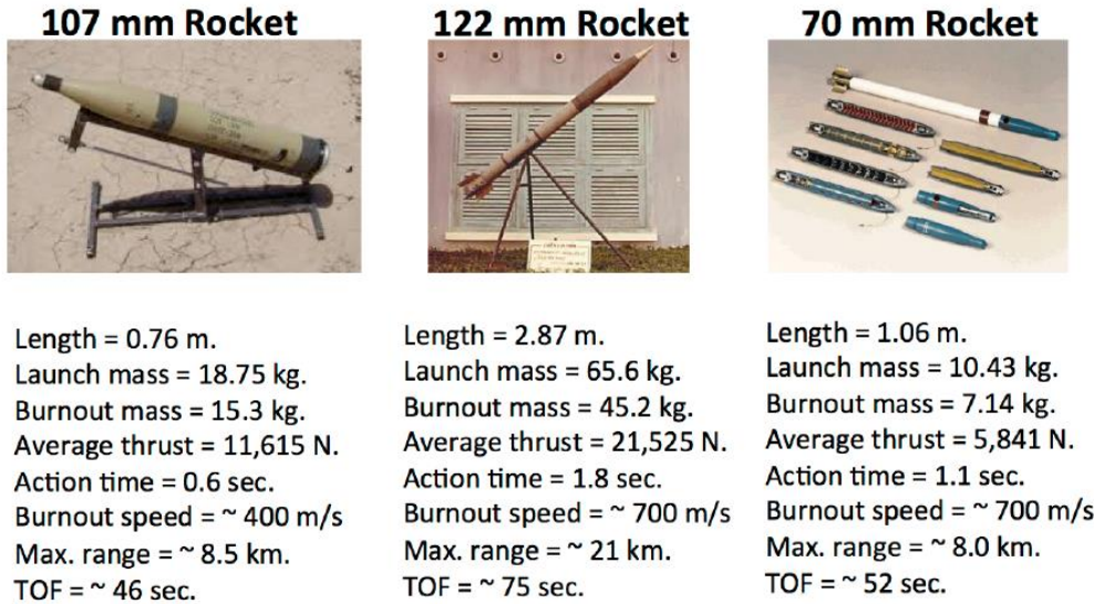
Figure 7: Description of Example Threat/Target Physical Parameters used in this paper. It is clear that the 70 mm and 107 mm rockets have similar physical characteristics, as well as, expected flight performances, but the 122 mm rocket is much bigger than both with typically longer -range and time of flight.
