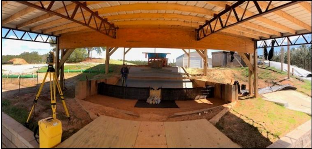
Figure 3.11. Robotic total station setup and survey.
