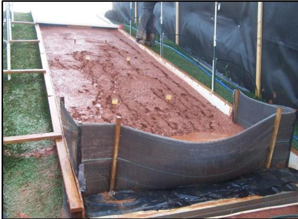
Figure 2.9. Modified ASTM D7351 test apparatus. ( Sprague and Sprague 2012 )
