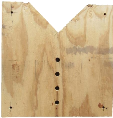
(a) plywood dewatering weir
