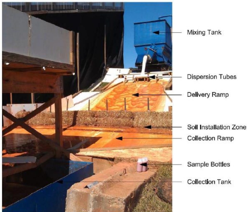
Figure 2.8. ASTM D7351 test apparatus. ( Troxel 2013 )
