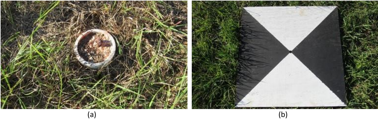
Figure 7.3. Image georeferencing: (a) control/check point; (b) ground target.
